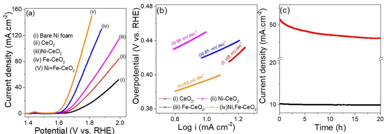
Fig. 7 (a) OER LSV curves (b) Tafel slope for OER, (c) OER *i-t* tests.
