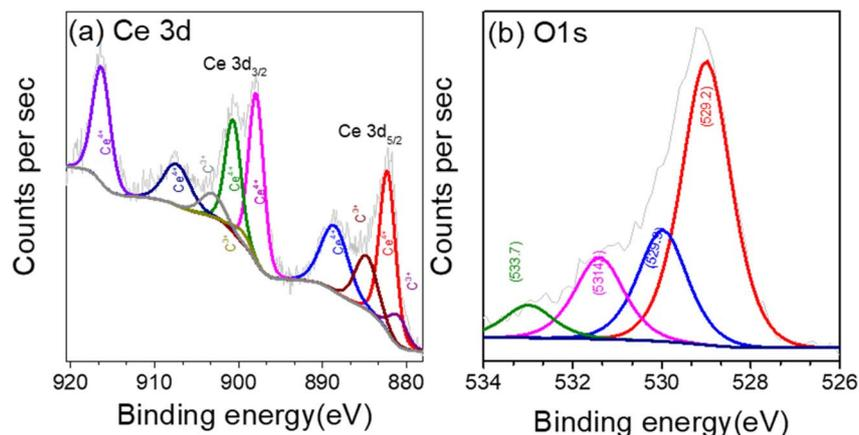
Fig. 5 (a) Region XPS spectra of CeO<sub>2</sub> nanoparticles (a) Ce 3d (b) O 1s.
