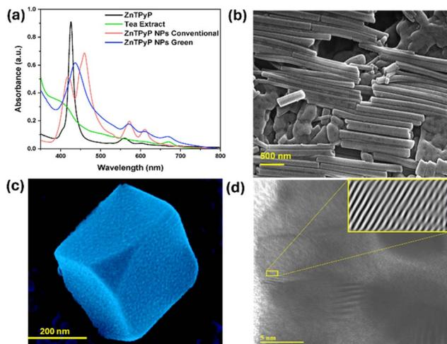
Fig. 1 Characterization data of porphyrinic nanoparticles (a) UV-vis absorption spectra of ZnTPyP, green tea extract, ZnTPyP-NRs synthesized *via* conventional method and ZnTPyP-NCs synthesized *via* bioinspired route. (b) FESEM image of CS-ZnTPyP-NRs. (c) FESEM image of GS-ZnTPyP-NC. (d) HRTEM image of bioinspired GS-ZnTPyP-NCs.
