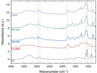
Fig. 7 Comparison of FTIR spectra for the initial oxidized MND, the size sorted ones collected from the 10% EG and 40% EG layers and pellet. An EG reference was added for comparison.
