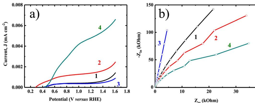
Fig. 5 (a) LSV and (b) Nyquist plot of anatase granular (1-dark 2-light) and rutile TiO<sub>2</sub> nanorod (3-dark 4-light).
