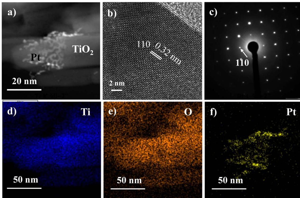
Fig. 7 (a) ADF STEM image of rutile  $\text{TiO}_2$  nanorod after Pt deposition. (b) HRTEM image taken on the surface of rutile  $\text{TiO}_2$  particle (c) SAED pattern for the rutile  $\text{TiO}_2$  particle, confirming the formation of a single crystal and (d–f) elemental mapping for Ti, O, and Pt, respectively.
