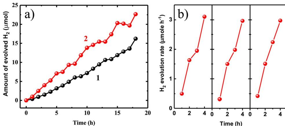
Fig. 6 (a) Photocatalytic H<sub>2</sub> generation under 300 W Xe-lamp for (1) anatase granular and (2) rutile TiO<sub>2</sub> nanorod, (b) three consecutive runs until maximum rate of H<sub>2</sub> generation.
