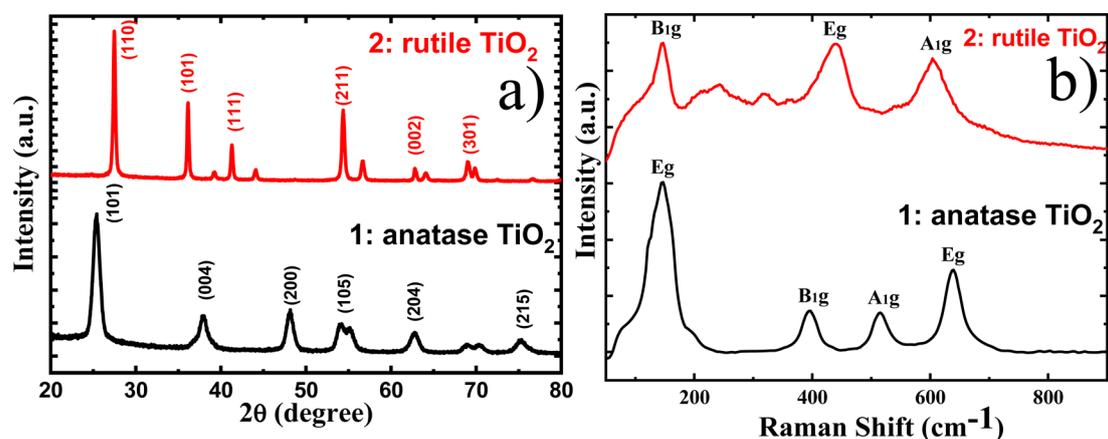
Fig. 2 (a) XRD pattern and (b) Raman spectra of anatase granular (1) and rutile  $\text{TiO}_2$  nanorod (2).
