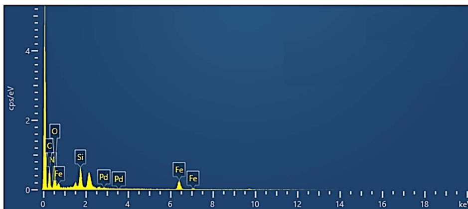
Fig. 11 EDS spectrum of the recovered \text{Fe}_3\text{O}_4/\text{GO-IL-Pd} catalyst.
