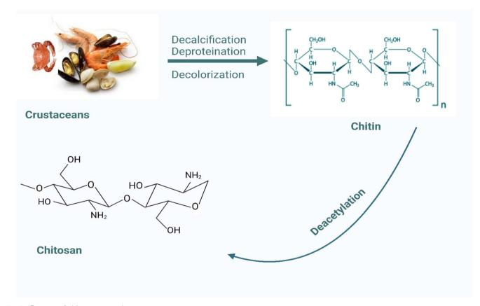
Fig. 3 Process of chitosan extraction.
