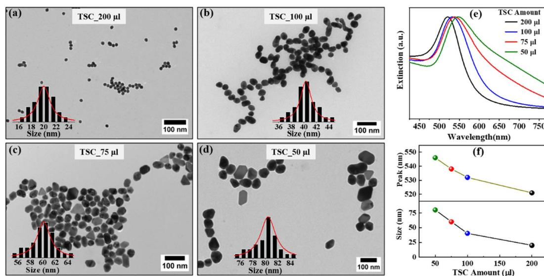
Fig. 1 TEM images of synthesized Au NPs with TSC amounts of (a)  $200\text{ }\mu\text{L}$ , (b)  $100\text{ }\mu\text{L}$ , (c)  $75\text{ }\mu\text{L}$ , and (d)  $50\text{ }\mu\text{L}$ . (e) the extinction spectra of Au NPs synthesized with different amounts of TSC, and (f) the plots showing the variations of size and SPR peak position of NPs with respect to the TSC amount.
