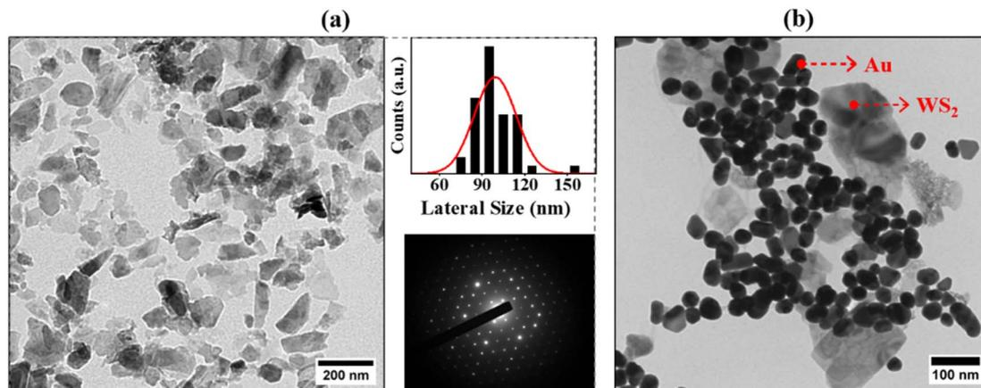
Fig. 4 (a) TEM image, lateral size distribution histogram, and SAED patterns of WS<sub>2</sub> nanoflakes, and (b) TEM image of nanohybrids.
