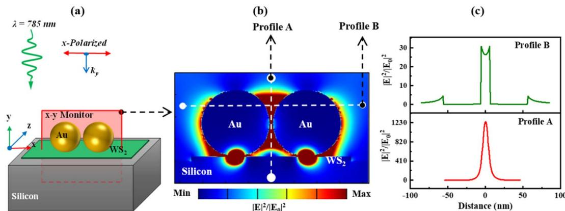
Fig. 7 (a) FDTD simulation structure of the two-particle system on WS<sub>2</sub>/Si substrate, (b) field-intensity enhancement profile around the NPs, and (c) the field-intensity line profiles simulated across the horizontal and vertical directions of the plasmonic hotspot.
