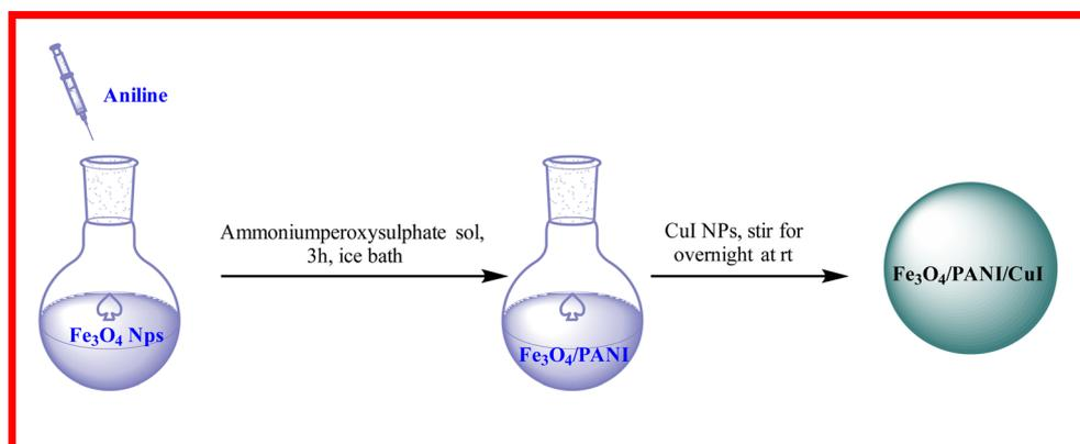
Fig. 2 Schematic diagram for the synthesis of nanocomposite.
