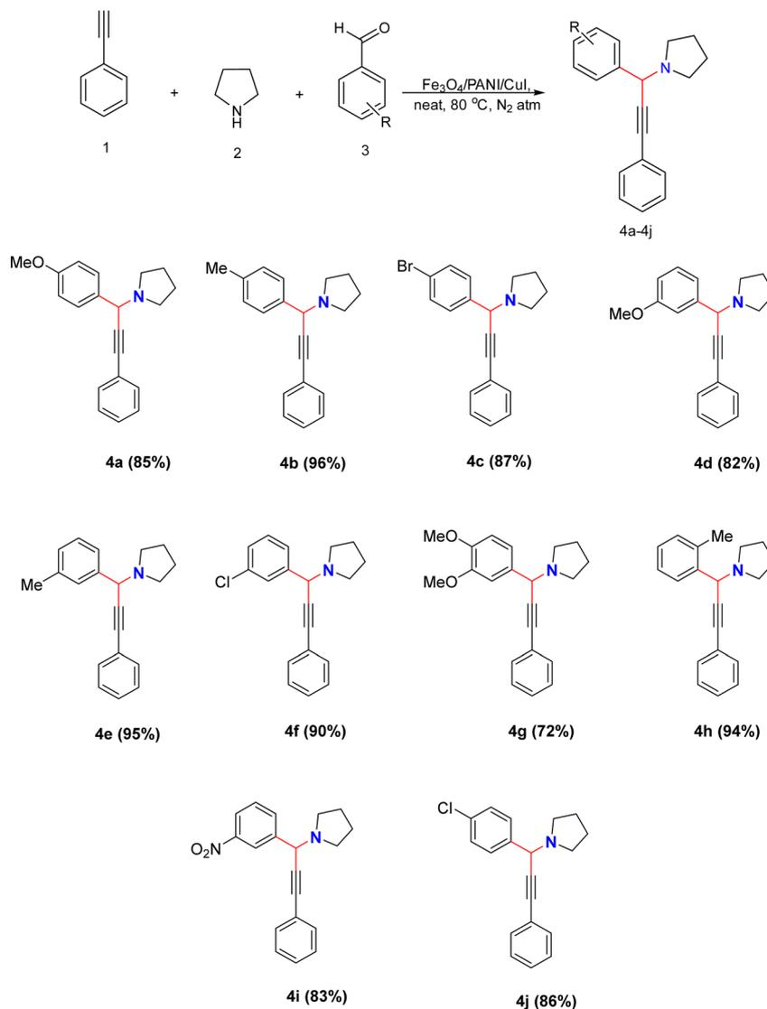
Scheme 1  $Fe_3O_4/PANI/CuI$  catalysed synthesis of propargyl derivatives via  $A^3$  coupling. Reaction conditions: nanocatalyst (10 mg), phenylacetylene (1 mmol), pyrrolidine (1 mmol), aromatic aldehyde (1 mmol), neat, 80 °C,  $N_2$  atm, 10 min.
