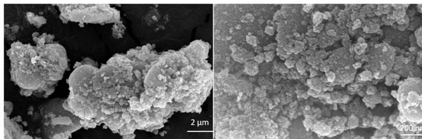
Fig. 4 FESEM analysis of Fe<sub>3</sub>O<sub>4</sub>/PANI/CuI nanocatalyst.
