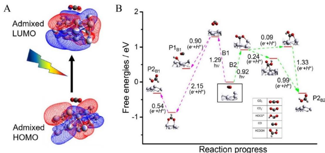
Fig. 14 The mechanism of photocatalytic CO<sub>2</sub> reduction, derived from Density Functional Theory (DFT) calculations, is outlined as follows: (A) examination of the Highest Occupied Molecular Orbital (HOMO) and Lowest Unoccupied Molecular Orbital (LUMO) of the CO<sub>2</sub>/Ag complex; (B) identification of potential reaction pathways.<sup>176</sup>
