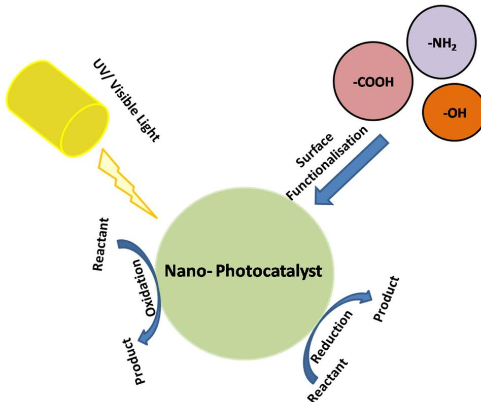
Fig. 6 Surface functionalization of nano-photocatalysts with  $\text{-COOH}$ ,  $\text{NH}_2$ , and  $\text{OH}$  groups to enhance their reactivity.
