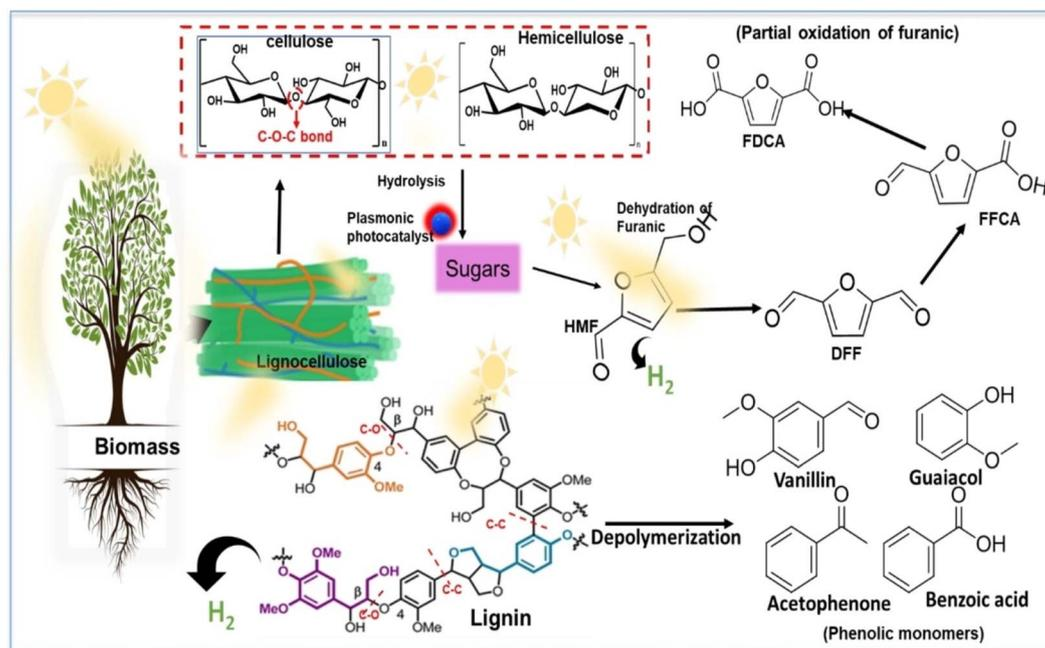
Fig. 15 Schematic diagram illustrating the pathways for photocatalytic conversion of lignocellulose biomass (LCB) into valuable chemicals and hydrogen gas. Key compounds involved in the process include 2,5-diformylfuran (DFF), 2,5-furandicarboxylic acid (FDCA), and 5-hydroxymethylfurfural (HMF).<sup>155</sup>
