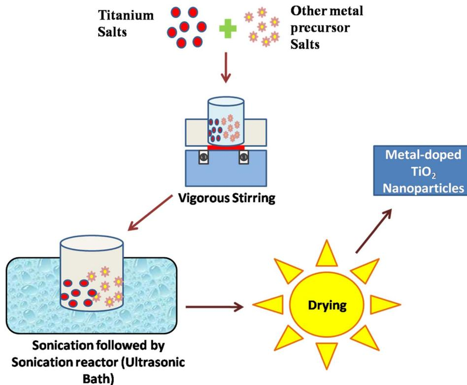
Fig. 10 Flow chart for the preparation of metal-doped TiO<sub>2</sub> plasmonic nanoparticles via the sonochemical method.
