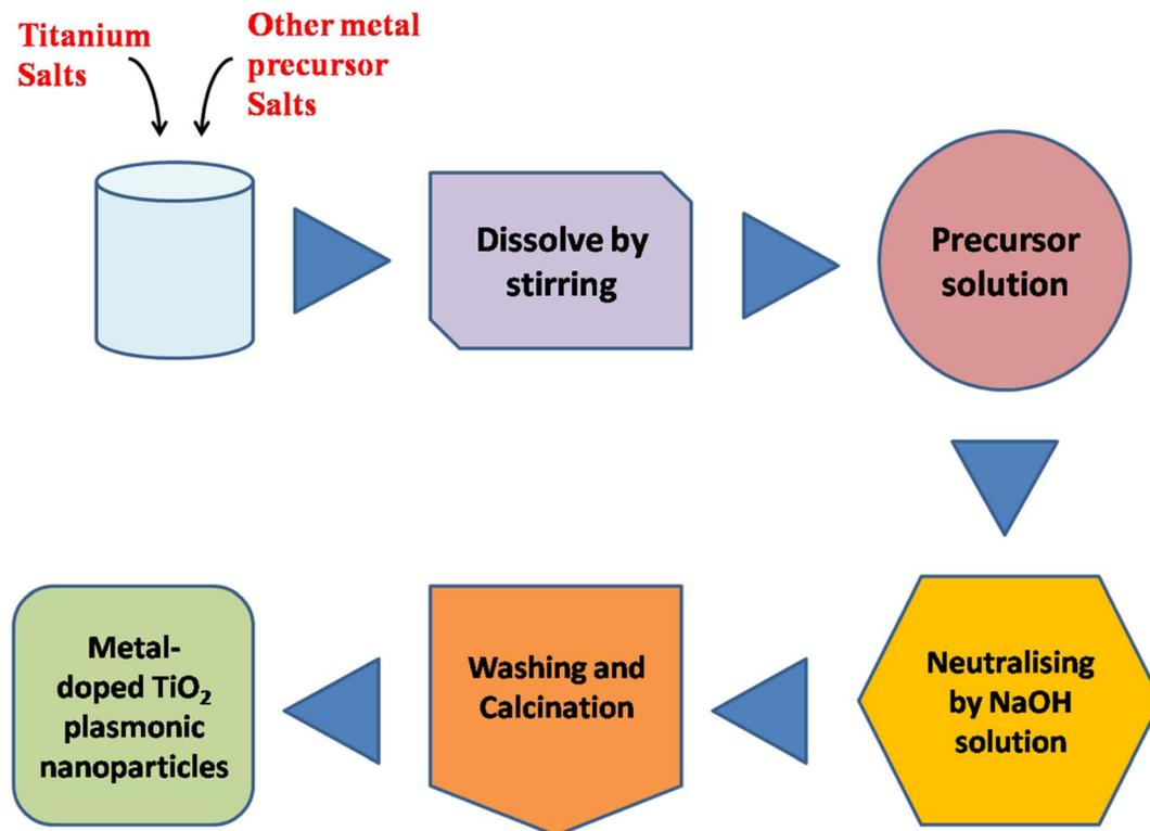
Fig. 9 Deposition–precipitation method for the synthesis of metal-doped TiO<sub>2</sub> nanomaterials.
