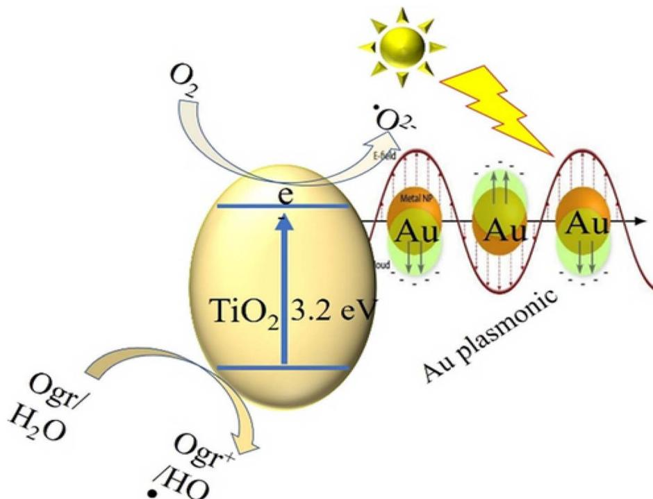
Fig. 8 Au doped  $\text{TiO}_2$  nano-photocatalyst. Adapted from Copyright JCCS, Wiley 2021.<sup>96</sup>
