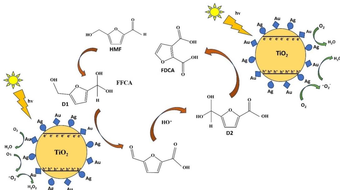
Fig. 11 Mechanism behind photocatalytic oxidation of HMF to FDCA using the Ag–Au/TiO<sub>2</sub> photocatalyst.
