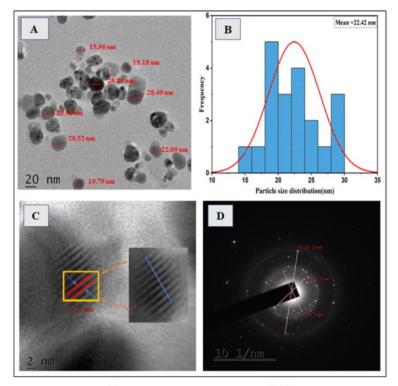
Fig. 5 (A) HR-TEM image of the Hc-AgNPs, (B) histogram plot of the Hc-AgNPs from figure (A), (C) lattice fringes at higher resolution of the Hc-AgNPs, and (D) SAED pattern of the Hc-AgNPs.
