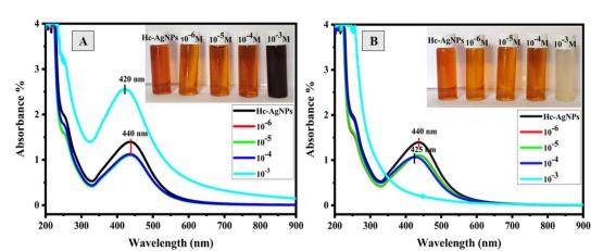
Fig. 8 UV-visible spectra of Hc-AgNPs as a function of various concentrations of (A) Sn<sup>2+</sup> and (B) Hq<sup>2+</sup> ions
