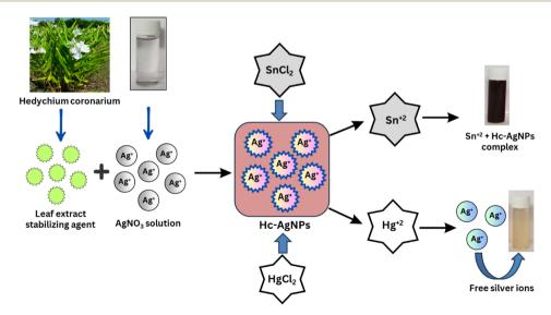
Fig. 9 Possible interaction mechanism of Hc-AgNPs with Sn<sup>2+</sup> and Hg<sup>2+</sup> ions.
