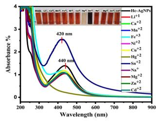
Fig. 7 UV-visible absorbance spectra of Hc-AgNPs with supplemented metal ions and the selective sensing of  $\rm Sn^{2+}$  and  $\rm Hg^{2+}$  metal ions by Hc-AgNPs in an aqueous medium.
