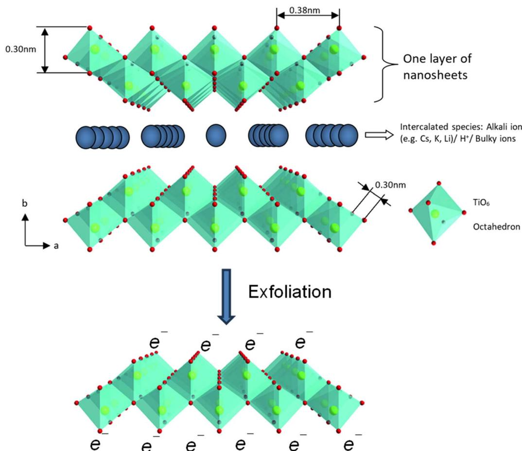
Fig. 11 The polyhedral representation of the crystal structure of layered lepidocrocite-like titania nanosheets viewed down along the *c*-axis and mono-layer titania nanosheets after exfoliation. Adapted from ref. 88 with permission from the Royal Society of Chemistry.
