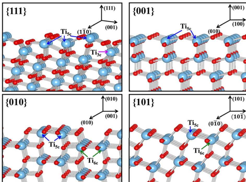
Fig. 10 Slab model for the surface structures of the relaxed stoichiometric  $\text{TiO}_2$ 's  $\{111\}$ ,  $\{001\}$ ,  $\{010\}$  and  $\{101\}$  facets. Reprinted with permission from ref. 100. Copyright ©2013, American Chemical Society.
