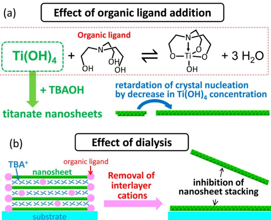
Fig. 7 The illustration of (a) the effect of the organic ligand in the crystallisation of the titania nanosheets and (b) inhibition of nanosheets restacking by dialysis.<sup>87</sup> Copyright © 2015, American Chemical Society.
