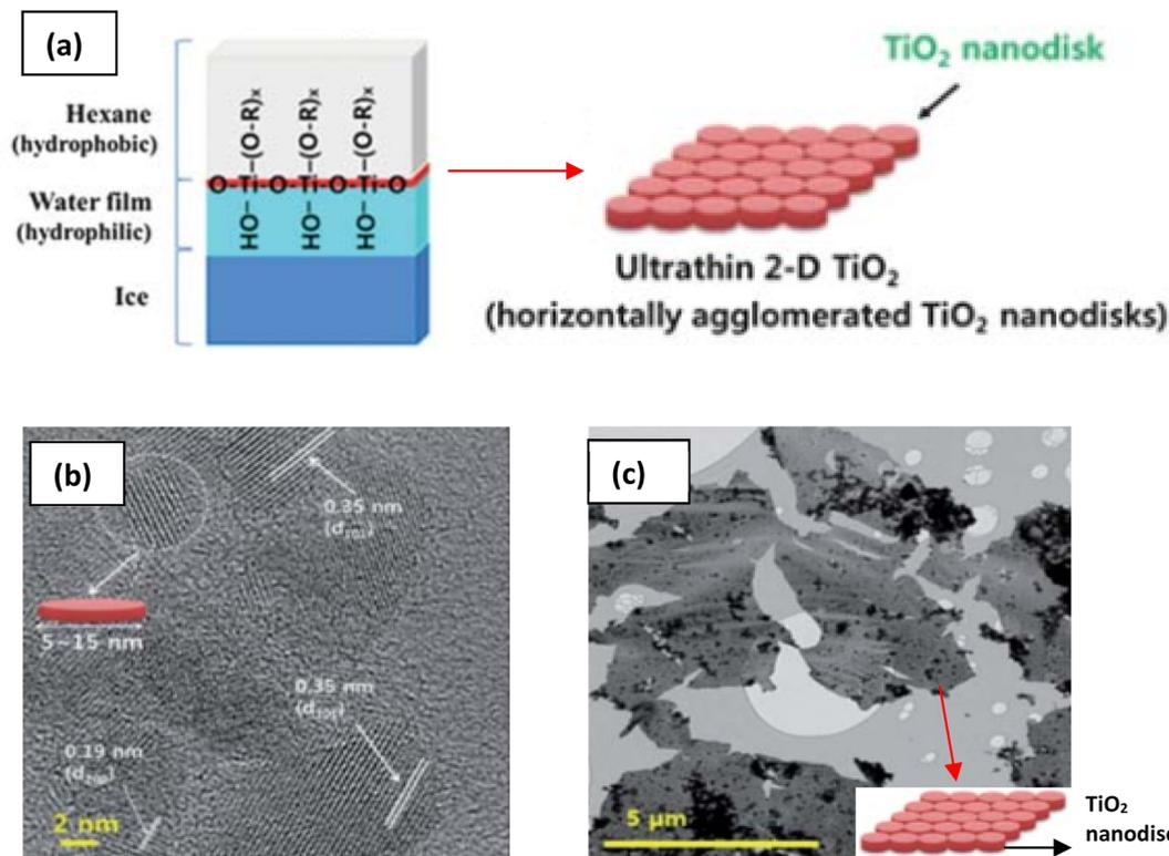
Fig. 8 (a) Schematic illustration of the 2-D  $\text{TiO}_2$  formation on the hexane/ice interface.<sup>84</sup> TEM images of a nanosheet consisting of horizontally agglomerated  $\text{TiO}_2$  nanodisks.<sup>84</sup> (b) HR-TEM image of nanodisks, (c) TEM image of nanosheets. Reproduced from ref. 84 with permission from the Royal Society of Chemistry.
