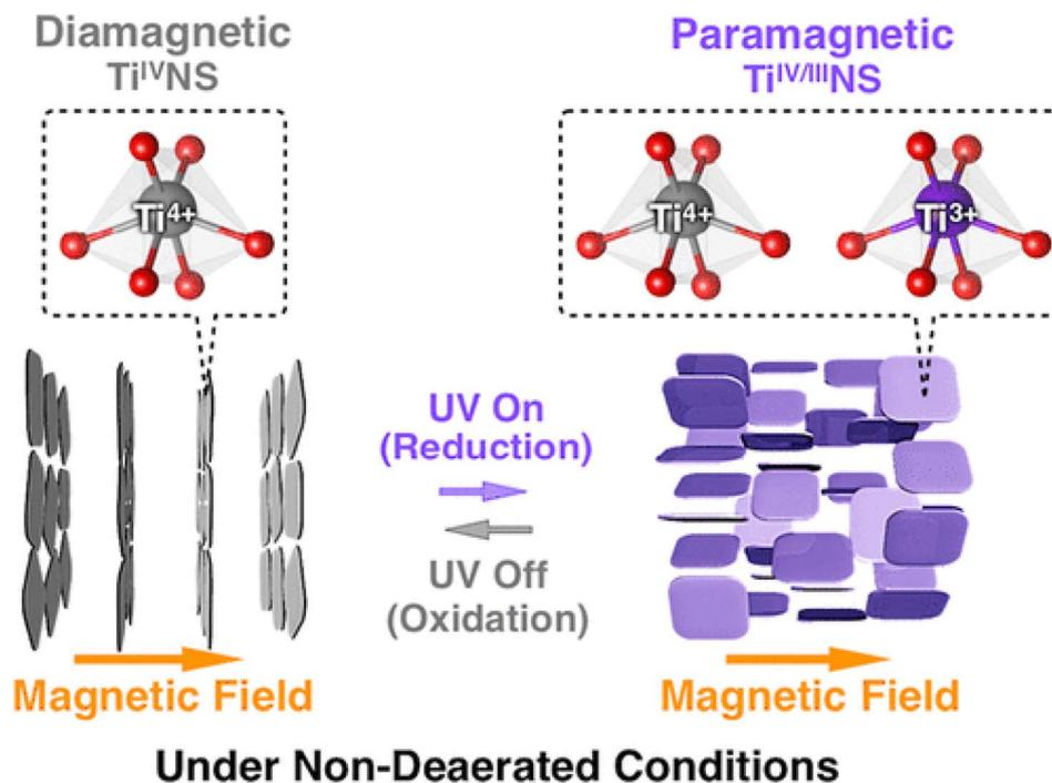
Fig. 12 The orthogonal and parallel magnetic orientation switching of titania nanosheets *via* photoreduction and oxidation.<sup>118</sup> Copyright © 2018, American Chemical Society.
