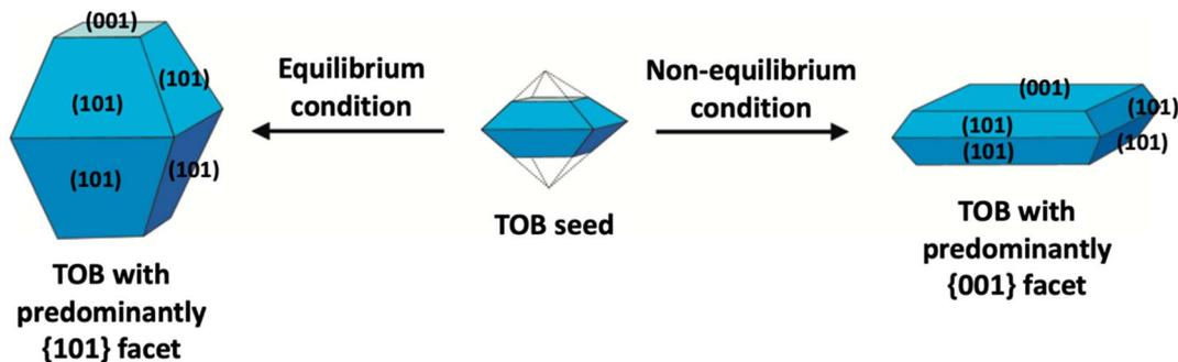
Fig. 3 Schematic illustration of the  $\text{TiO}_2$  crystal evolution under equilibrium and non-equilibrium conditions.
