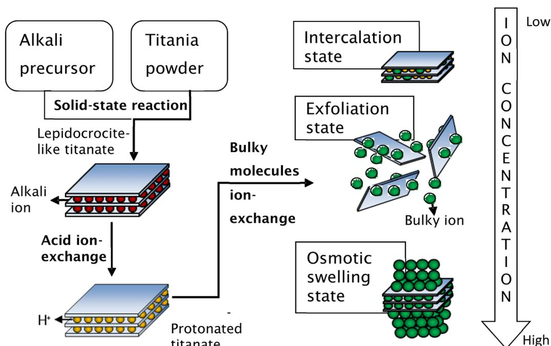
Fig. 6 Schematic representation of the synthesis of single-layer titania nanosheets *via* chemical exfoliation process.<sup>80</sup> Copyright © 2017 IOP Publishing.
