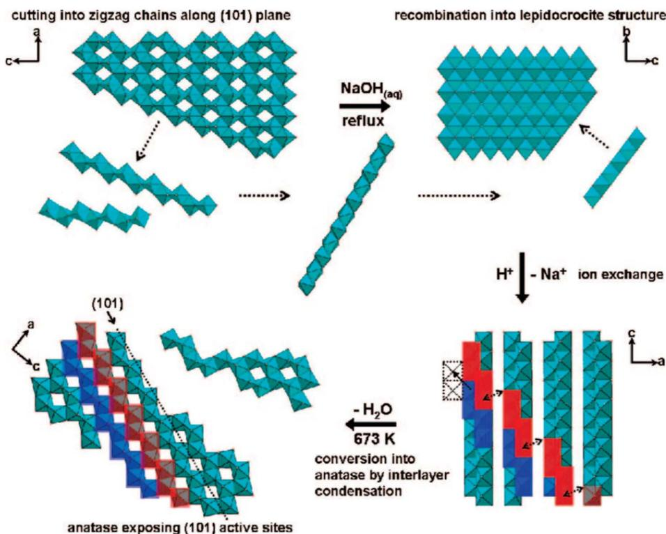
Fig. 2 Schematic illustration of the conversion pathway of commercial bulk anatase to two-dimensional (101)-exposed anatase TiO<sub>2</sub> nanosheet in the chimie-douce method. Reprinted with permission from ref. 48. Copyright 2008, American Chemical Society.
