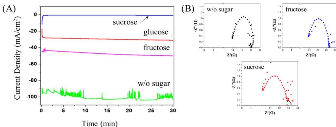
Fig. 3 Current density as a function of reaction time during the electrochemical reduction of sugars in the presence of  $\text{H}_2\text{O}_2$  (A) and the charge transfer resistance ( $R_{ct}$ ) on electrochemical reduction of sugars (B) in comparison to the reaction in the absence of sugar.
