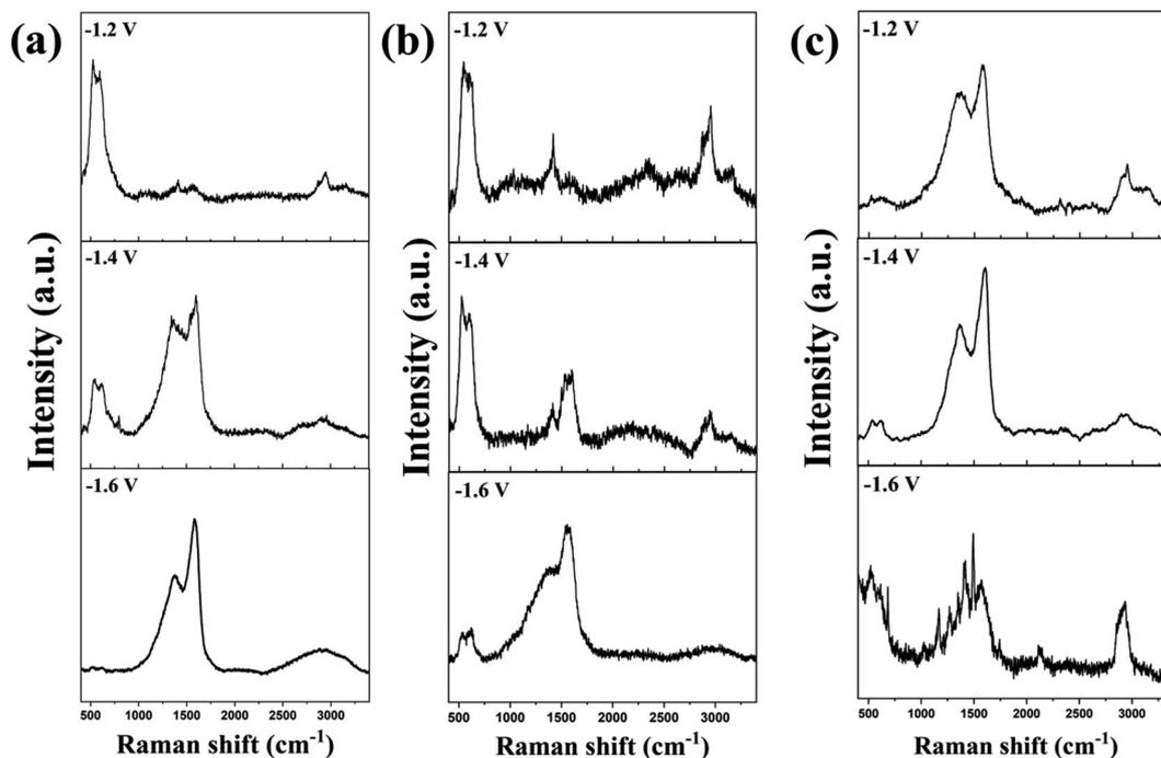
Fig. 6 Raman spectra of the Ag/Cu electrocatalyst after electrochemical reduction of fructose (a), glucose (b), and sucrose (c) at different applied potentials vs. Ag/AgCl.
