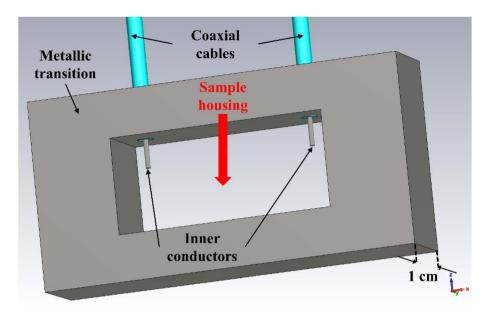
EM layout of the metallic transition used to apply an external DC bias voltage to a DUT placed inside the X-band waveguides.
