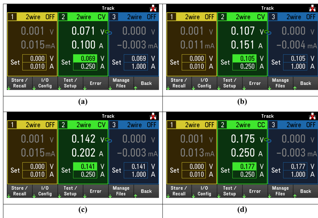
Fig. 11 Screenshots of the voltage source with different voltage–current combinations applied to the sample of fused silica with sample C. From (a) to (d), the resistance slowly decreases from 0.71 to 0.7 \Omega .
