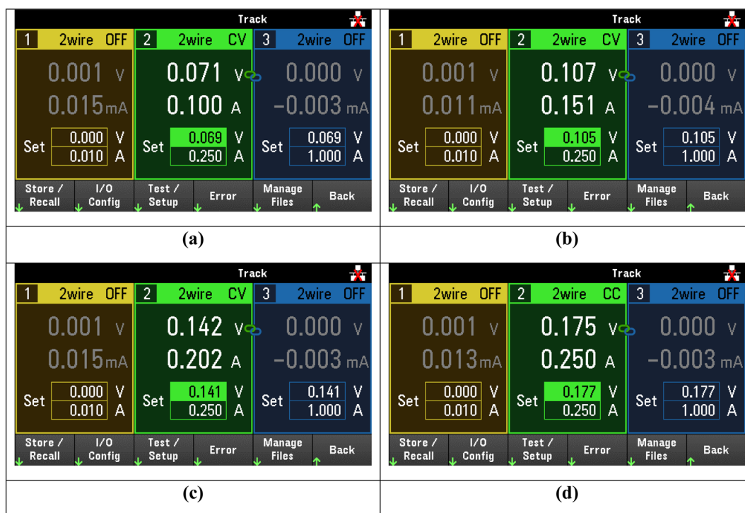
Fig. 11 Screenshots of the voltage source with different voltage–current combinations applied to the sample of fused silica with sample C. From (a) to (d), the resistance slowly decreases from 0.71 to 0.7 \Omega .
