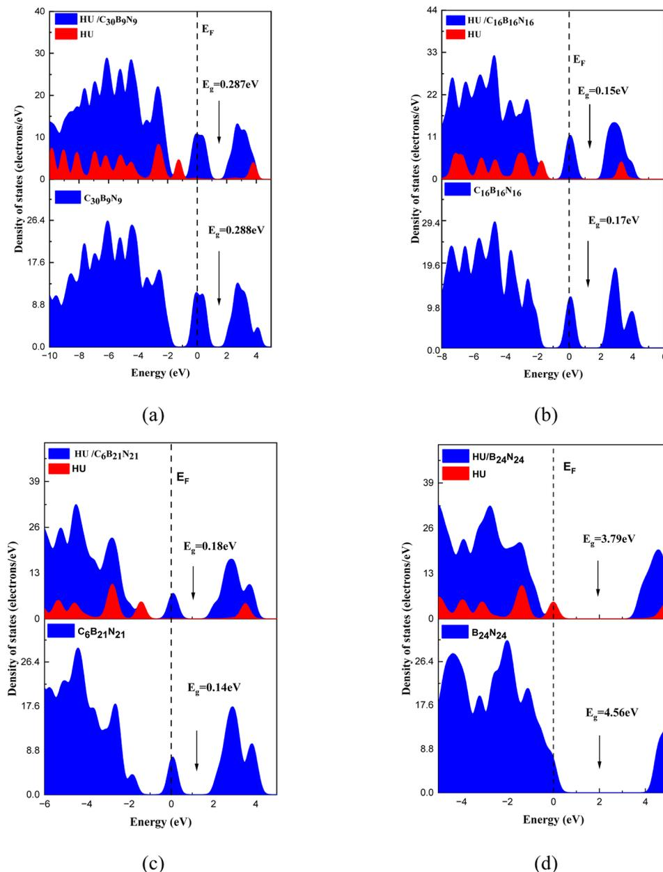
Fig. 4 DOS and PDOS spectra of the pristine, doped nanosheets, and their complexes: (a)  $C_{30}B_9N_9$ , (b)  $C_{16}B_{16}N_{16}$ , (c)  $C_6B_{21}N_{21}$ , and (d)  $B_{24}N_{24}$ .
