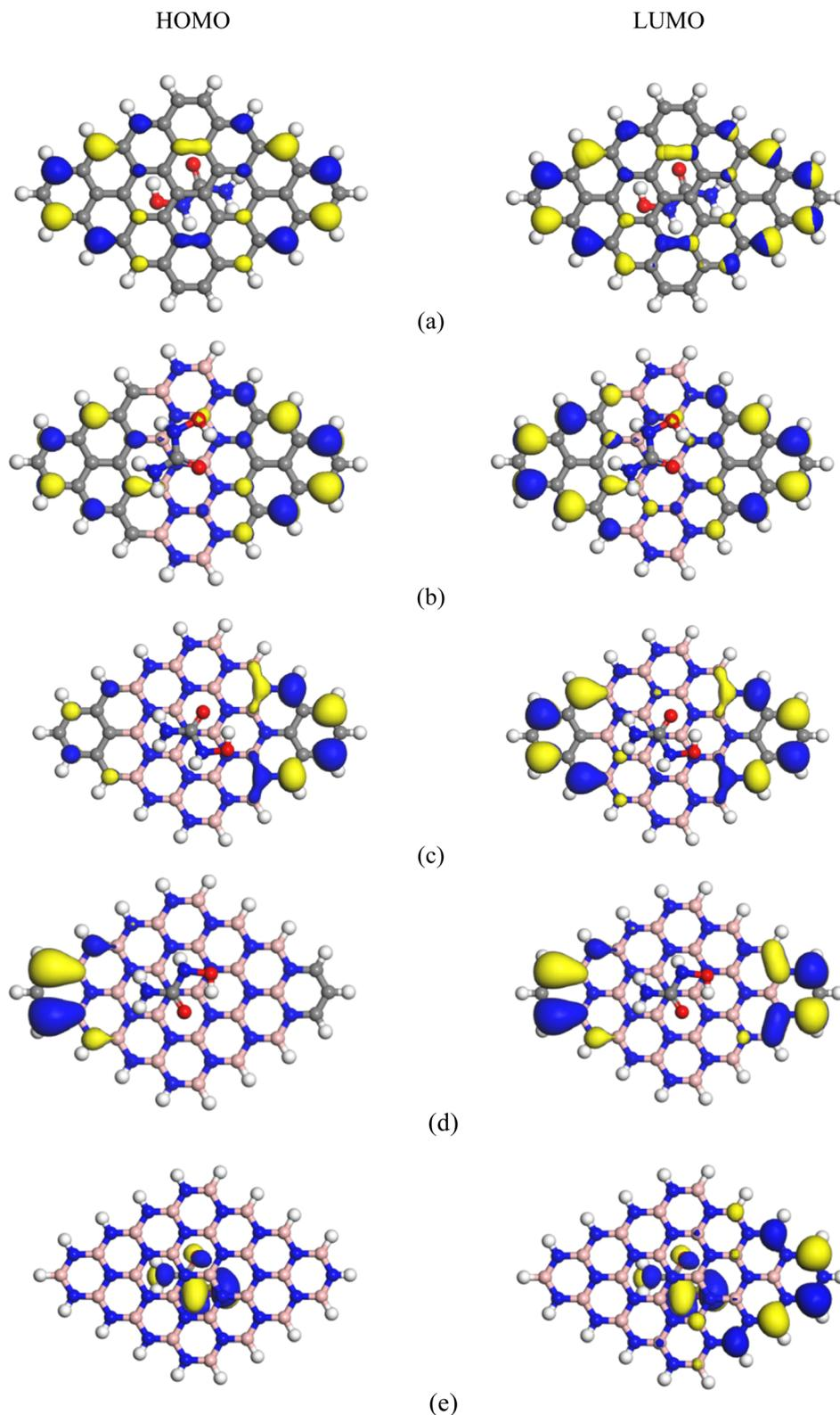
Fig. 3 HOMO and LUMO maps of the complexes: (a) HU/C<sub>48</sub>, (b) HU/C<sub>30</sub>B<sub>9</sub>N<sub>9</sub>, (c) HU/C<sub>16</sub>B<sub>16</sub>N<sub>16</sub>, (d) HU/C<sub>6</sub>B<sub>21</sub>N<sub>21</sub>, and (e) HU/B<sub>24</sub>N<sub>24</sub>.
