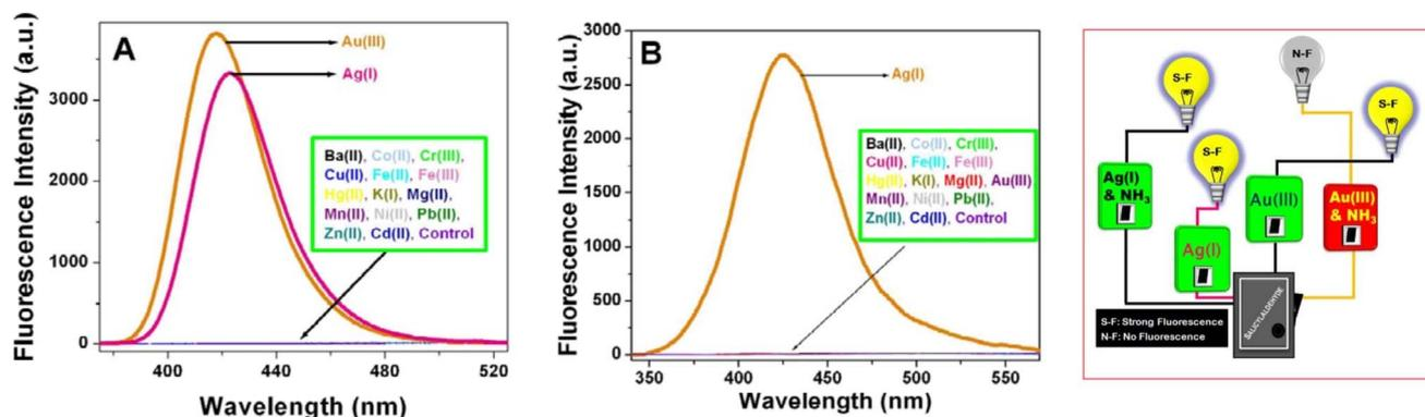
Fig. 6 Displayed imine brings selectivity for silver-enhanced fluorescence (A) without imminic bond, (B) with imminic bonds. Reproduced with permission from ref. 32, copyright 2024, *Dalton Trans.*
