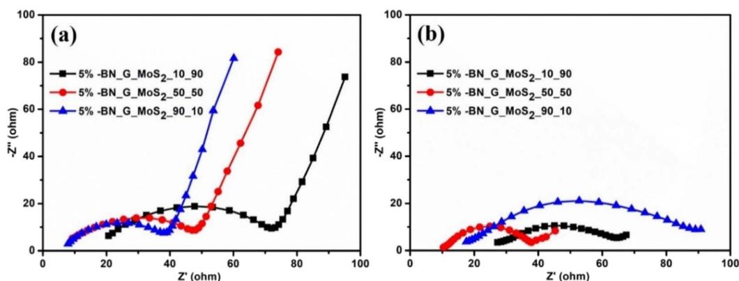
Fig. 7 Electrochemical impedance spectroscopy spectra of the as-fabricated (a) and after 150 cycles (b) of the 5% BN-G@MoS<sub>2</sub>-10@90, 5% BN-G@MoS<sub>2</sub>-50@50 and 5% BN-G@MoS<sub>2</sub>-90@10 anodes.
