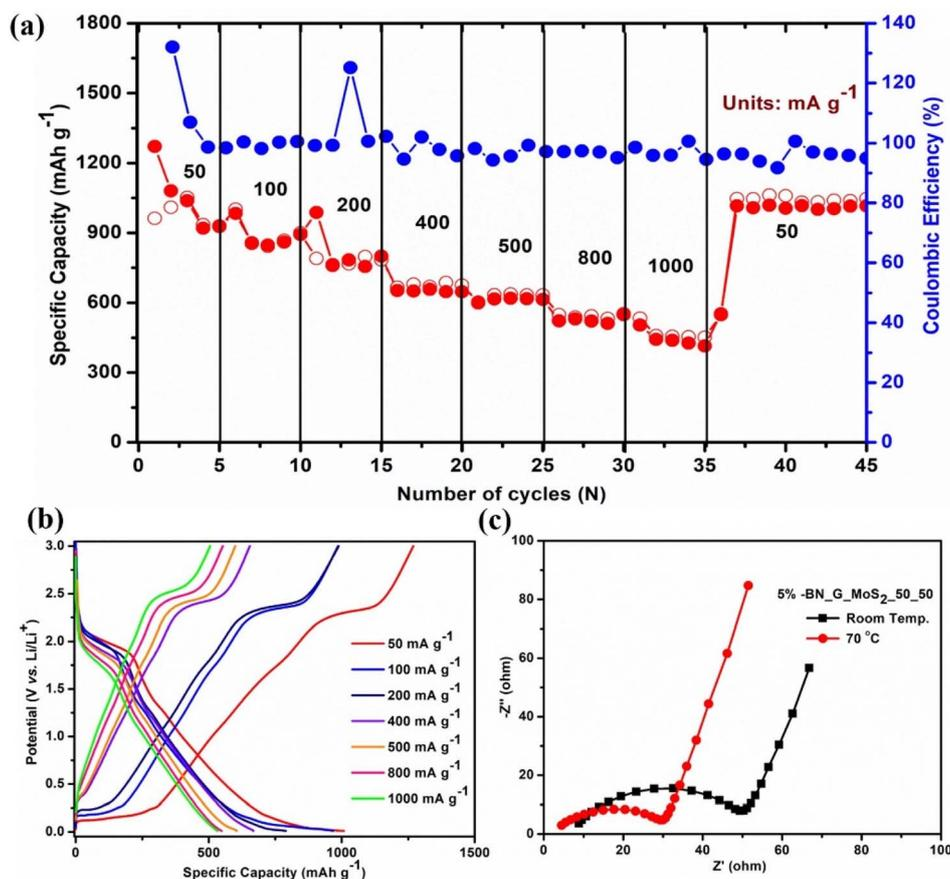
Fig. 8 (a) Rate performance, (b) galvanostatic discharge–charge curves at high temperature and (c) Nyquist plot at room temperature and high temperature of the 5% BN-G@MoS<sub>2</sub>-50@50 composite electrode.
