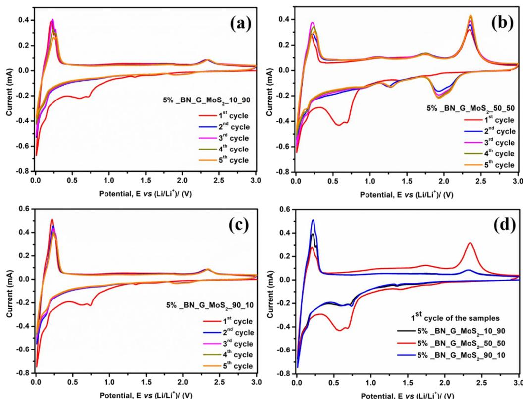
Fig. 4 (a–c) Cyclic voltammograms of 5% BN-G@MoS<sub>2</sub>-10@90, 5% BN-G@MoS<sub>2</sub>-50@50 and 5% BN-G@MoS<sub>2</sub>-90@10 anodes at a scan rate of 0.05 mV s<sup>-1</sup> and (d) 1st CV cycle curves of the 5% BN-G@MoS<sub>2</sub>-10@90, 5% BN-G@MoS<sub>2</sub>-50@50 and 5% BN-G@MoS<sub>2</sub>-90@10 anodes.
