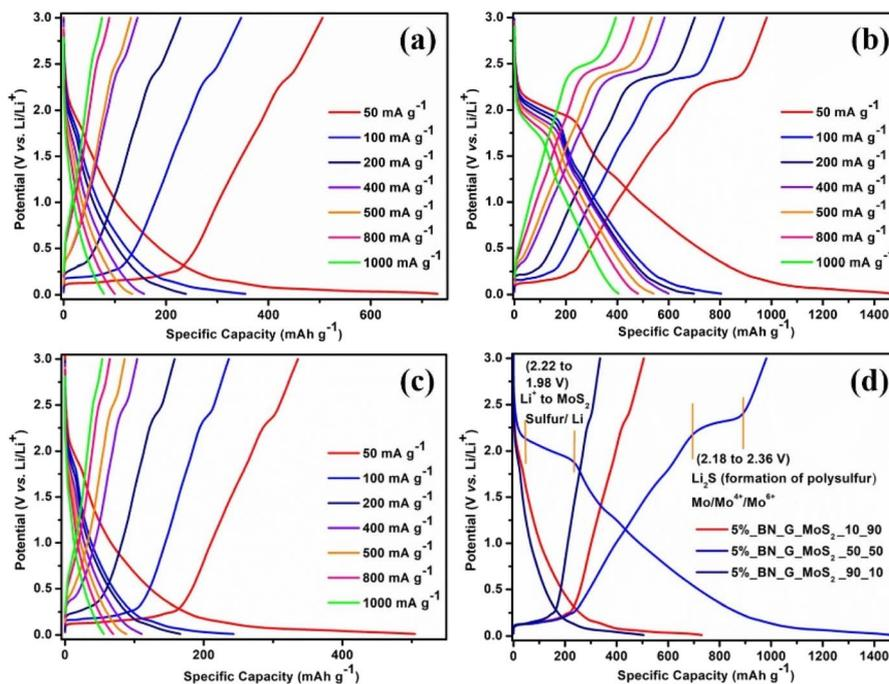
Fig. 6 Galvanostatic charge–discharge curves of (a) 5% BN-G@MoS<sub>2</sub>-10@90, (b) 5% BN-5% BN-G@MoS<sub>2</sub>-50@50, and (c) G@MoS<sub>2</sub>-90@10 composite electrodes at different current rates and (d) GCD curves of the three composites at 50 mA g<sup>-1</sup>.
