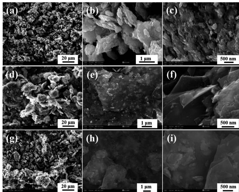
Fig. 2 SEM images of (a-c) 5% BN-G@MoS<sub>2</sub>-10@90, (d-f) 5% BN-G@MoS<sub>2</sub>-90@10 and (g-i) 5% BN-G@MoS<sub>2</sub>-50@50 materials.
