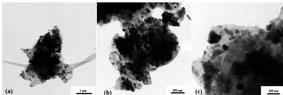
Fig. 3 TEM images of (a–c) 5% BN-G@MoS<sub>2</sub>-50@50 composite material.
