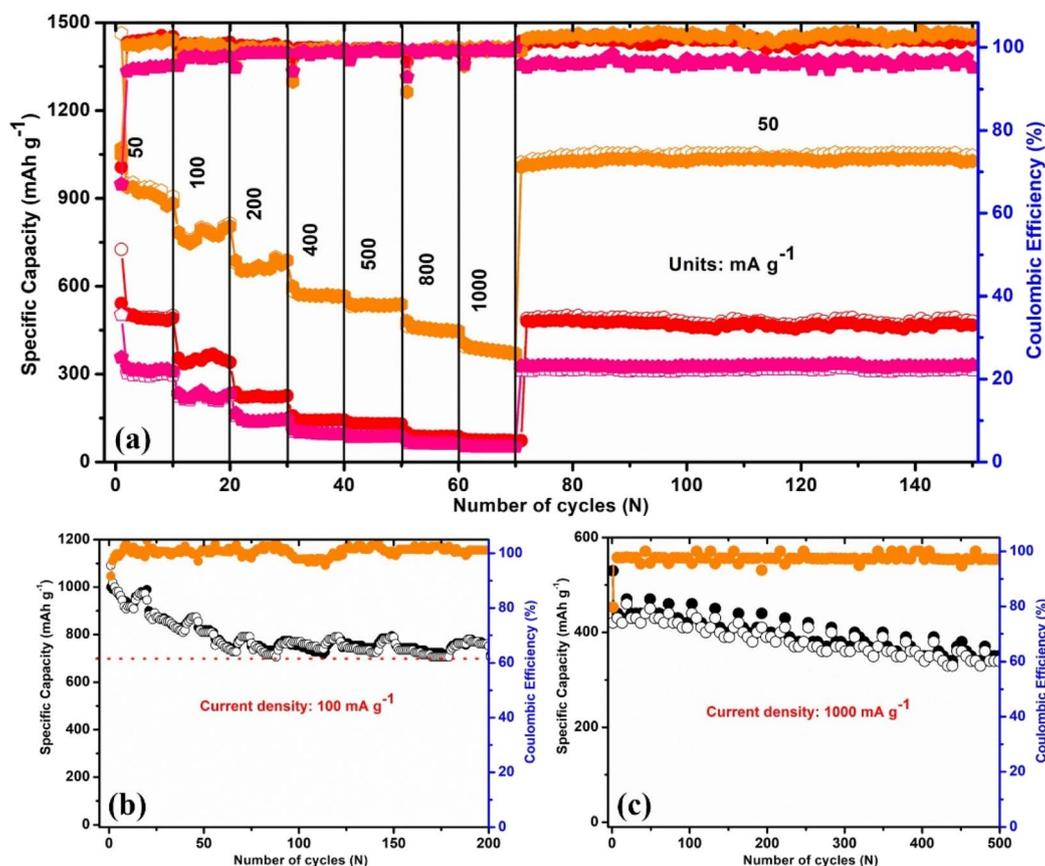
Fig. 5 (a) Rate capability (50 to 1000  $\text{mA g}^{-1}$ ) and long-term cycling performance at 50  $\text{mA g}^{-1}$  of 5% BN-G@ $\text{MoS}_2$ -10@90, 5% BN-G@ $\text{MoS}_2$ -50@50, and 5% BN-G@ $\text{MoS}_2$ -90@10 composite electrodes, and long-term cycling performance and coulombic efficiencies of the 5% BN-G@ $\text{MoS}_2$ -50@50 composite electrode tested at current densities of (b) 100  $\text{mA g}^{-1}$  and (c) 1000  $\text{mA g}^{-1}$ .
