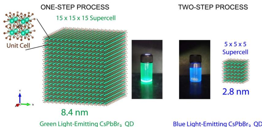
Fig. 1 CsPbBr<sub>3</sub> NCs with a cubic structure: green and blue-emitting NCs depending on the processing conditions: one-step vs. two-step. Unit-cell edge length is 0.587 nm.
