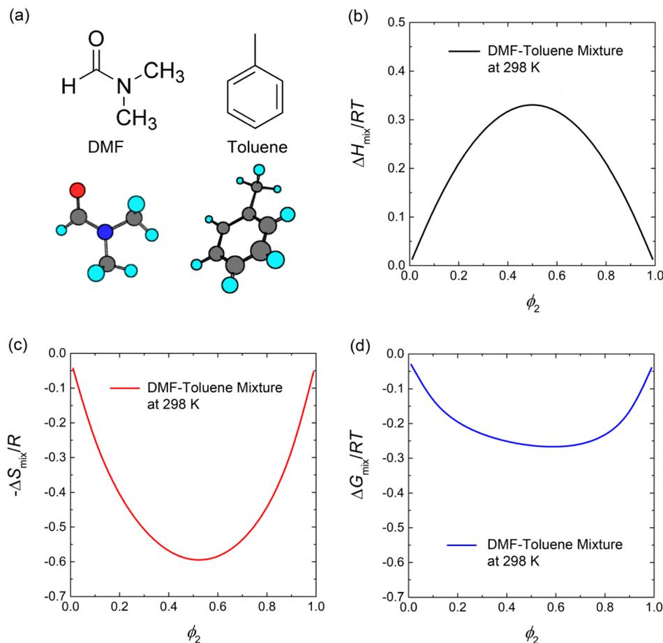
Fig. 3 (a) Chemical structures of DMF and toluene. Prediction of Flory–Huggins theory for (b) enthalpy of mixing, (c) entropy of mixing, and (d) Gibbs free energy of mixing as a function of volume fraction of toluene,  $\phi_2$  at 298 K.
