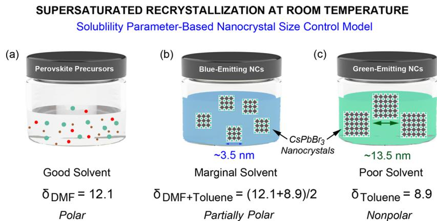
Fig. 11 Supersaturated recrystallization at room temperature: solubility parameter-based nanocrystal size control model: (a) good solvent = polar, (b) marginal solvent = partially polar, and (c) poor solvent or antisolvent = nonpolar.
