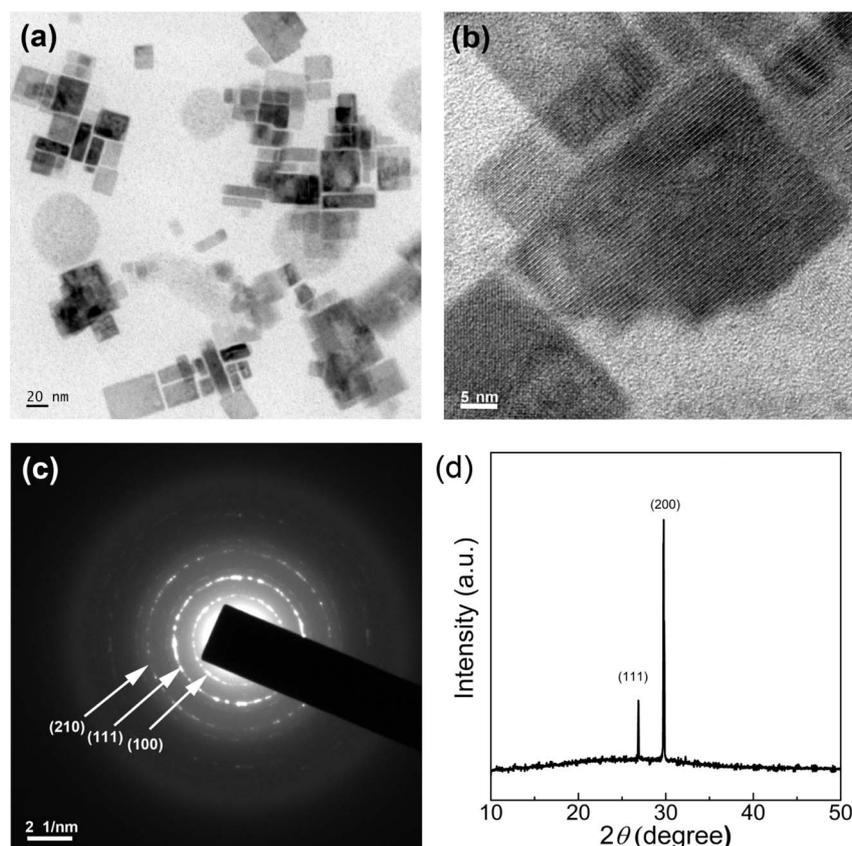
Fig. 8 TEM images of  $\text{CsPbBr}_3$  NCs synthesized through the two-step process with  $\text{CuBr}_2 : \text{PbBr}_2 = 1 : 4$  mole ratio: (a) scale bar = 20 nm, (b) scale bar = 5 nm, and (c) SAED image. (d) XRD pattern of  $\text{CsPbBr}_3$  NCs synthesized via a two-step process with  $\text{CuBr}_2 : \text{PbBr}_2 = 1 : 4$  mole ratio.
