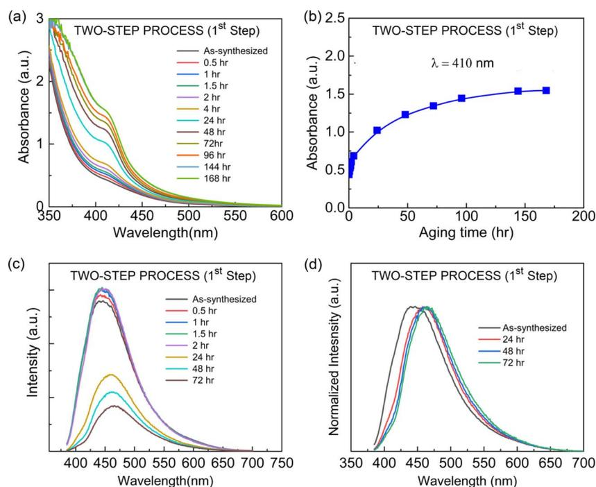
Fig. 10 Aging effect on the optical properties of CsPbBr<sub>3</sub> NCs (after the first step in the 'two-step process') at room temperature. (a) UV-vis absorption spectra as a function of aging time at room temperature. (b) The absorption at  $\lambda = 410$  nm. (c) PL emission spectra as a function of aging time at room temperature. (d) Normalized PL intensity as a function of aging time at room temperature.
