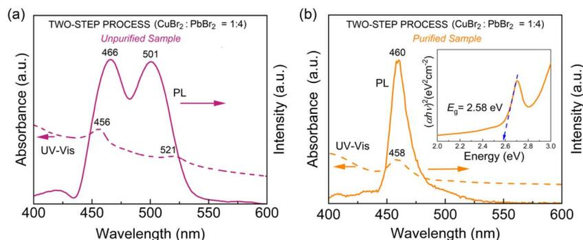
Fig. 9 UV-vis and PL spectra of CsPbBr<sub>3</sub> NCs synthesized through two-step synthesis with doping (CuBr<sub>2</sub> : PbBr<sub>2</sub> = 1 : 4 mole ratio): (a) unpurified sample and (b) purified sample. Inset: Tauc plot of the purified sample.
