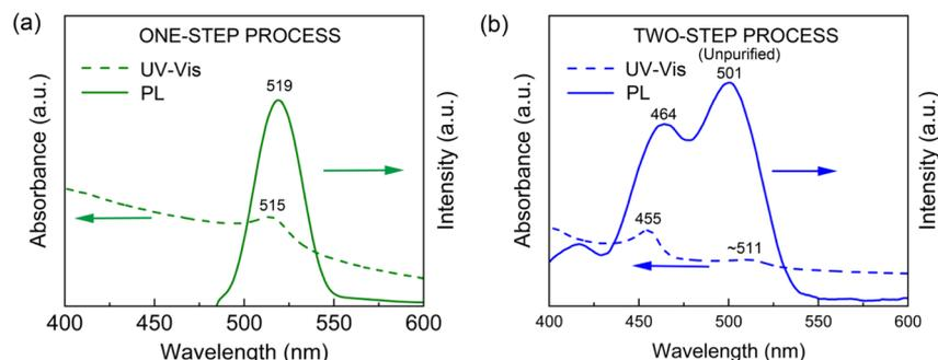
Fig. 6 UV-vis and PL spectra of CsPbBr<sub>3</sub> NCs: (a) one-step process and (b) two-step process without purification.
