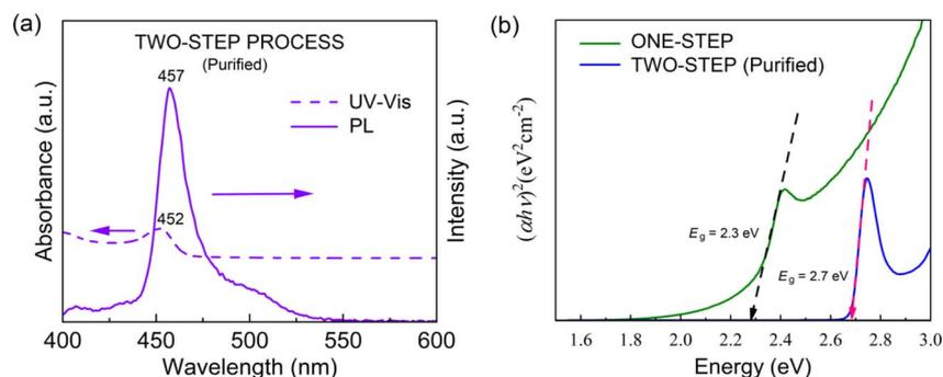
Fig. 7 (a) UV-vis and PL spectra for the purified two-step synthesized CsPbBr<sub>3</sub> NCs. (b) Tauc plot of one-step CsPbBr<sub>3</sub> NCs and two-step CsPbBr<sub>3</sub> NCs after purification.
