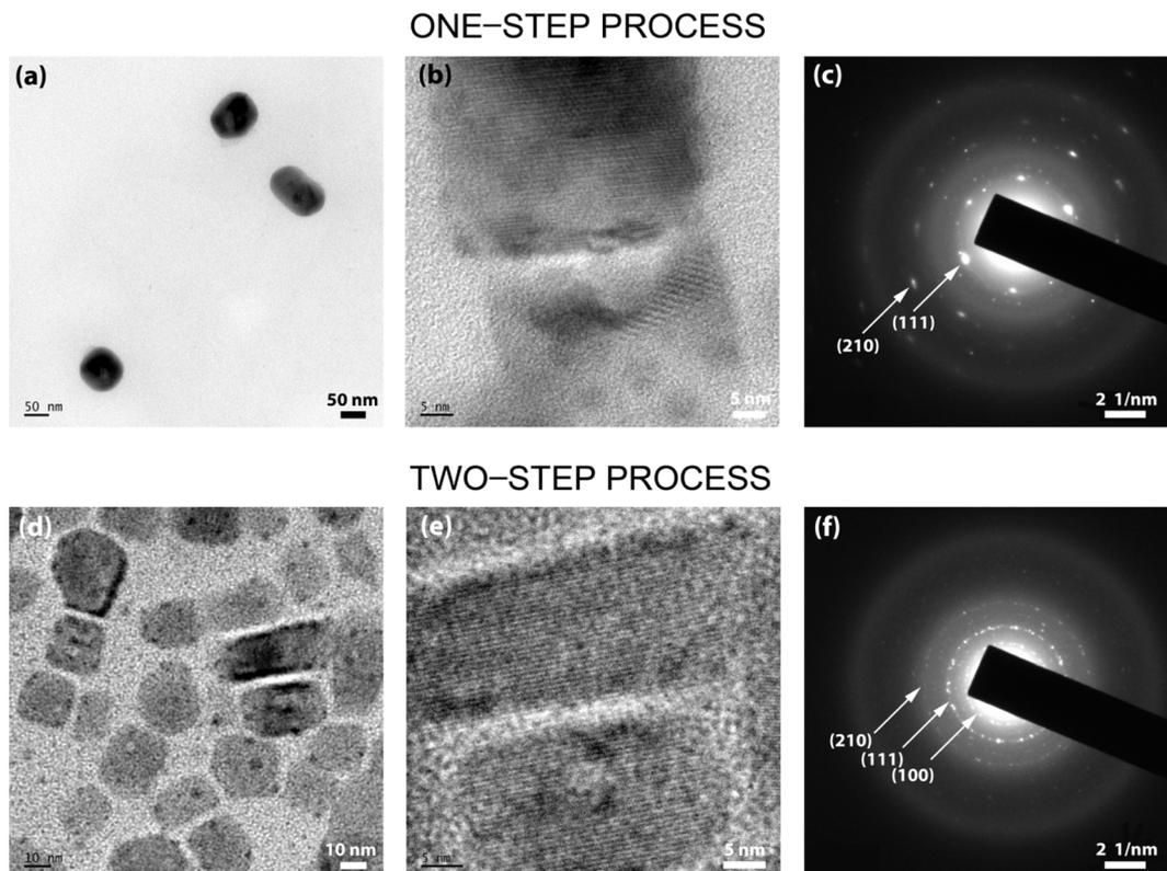
Fig. 4 TEM images of CsPbBr<sub>3</sub>NCs synthesized through (a and b) one-step synthesis and (d and e) two-step synthesis. SAED images: (c) one-step synthesis and (f) two-step synthesis.
