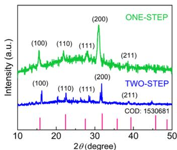
Fig. 5 XRD patterns of CsPbBr<sub>3</sub> NCs synthesized via the one-step and two-step SR method without purification.
