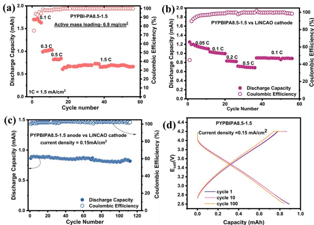
Fig. 5 (a) Rate studies and long cycling of the PYPBIPA8.5–1.5 based anodic half-cell at a high loading of  $6.8 \text{ mg cm}^{-2}$ ; (b) rate studies and (c) long cycling. (d) Charge discharge plots of PYPBIPA8.5–1.5 vs. the LiNCAO cathode full cell at  $0.15 \text{ mA cm}^{-2}$ .
