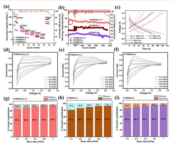
Fig. 3 (a) Comparison of the rate and (b) comparison of the long-cycling study results for 3000 cycles. (c) GCD curves for the 500th and 1000th cycles. (d–f) CV scan rate studies and (g-i) percentage contribution of diffusion-based and capacitive-based charge-storage currents for PYPBIPA8.5–1.5, 7–3 and 5–5, respectively.
