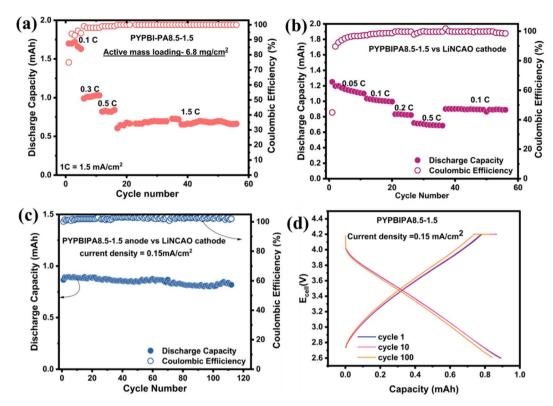
Fig. 5 (a) Rate studies and long cycling of the PYPBIPA8.5–1.5 based anodic half-cell at a high loading of 6.8 mg cm $^{-2}$ : (b) rate studies and (c) long cycling. (d) Charge discharge plots of PYPBIPA8.5–1.5 vs. the LiNCAO cathode full cell at 0.15 mA cm $^{-2}$ .
