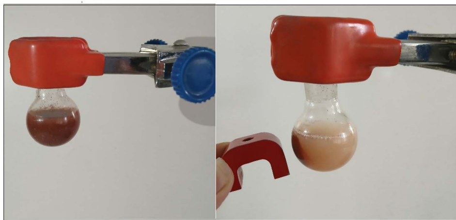
Fig. 7 Recyclability of Fe 3 O 4 @SiO 2 @SBA-3@2-ATP-Cu.
