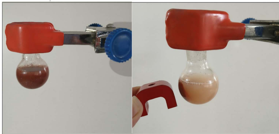
Fig. 7 Recyclability of Fe 3 O 4 @SiO 2 @SBA-3@2-ATP-Cu.
