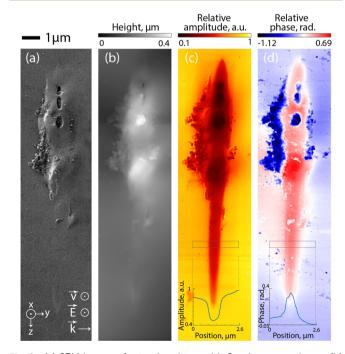
Fig. 2 (a) SEM image of a track written with 2 pulses per micron; (b) AFM surface topography; (c) 2D map of near-field scattered amplitude at  $1130~\rm cm^{-1}$ ; inset: cross-section profile indicating amplitude decrease across the laser track; (d) near-field phase map measured at  $1130~\rm cm^{-1}$ .
