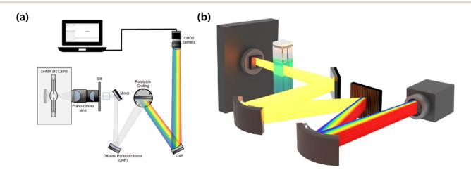
Fig. 5 (a) 2D and (b) 3D schematic images of real-time absorbance spectroscopy. The setup utilizes a broadband "white" light focused into a 100 μm vertical slit aperture via two plano-convex lenses. A light beam passing through the sample is collimated by an off-axis parabolic mirror (OAP) and is scattered upon encountering the grating. The scattering spectrum from the grating is recollimated by the second OAP mirror. The scattering spectrum from the grating is recorded by a CMOS camera.
