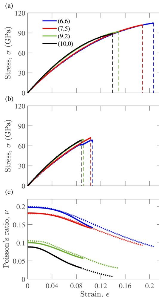
Fig. 3 Variation of stress ( $\sigma$ ) with strain ( $\epsilon$ ) curves for representative members of armchair, chiral, and zigzag configurations of (a) pristine and (b) defective (single vacancy) CNTs. (c) Variation of Poisson's ratio,  $\nu$  with strain,  $\epsilon$  for pristine and defective CNTs. The continuous and broken lines represent defective and pristine CNTs, respectively.
