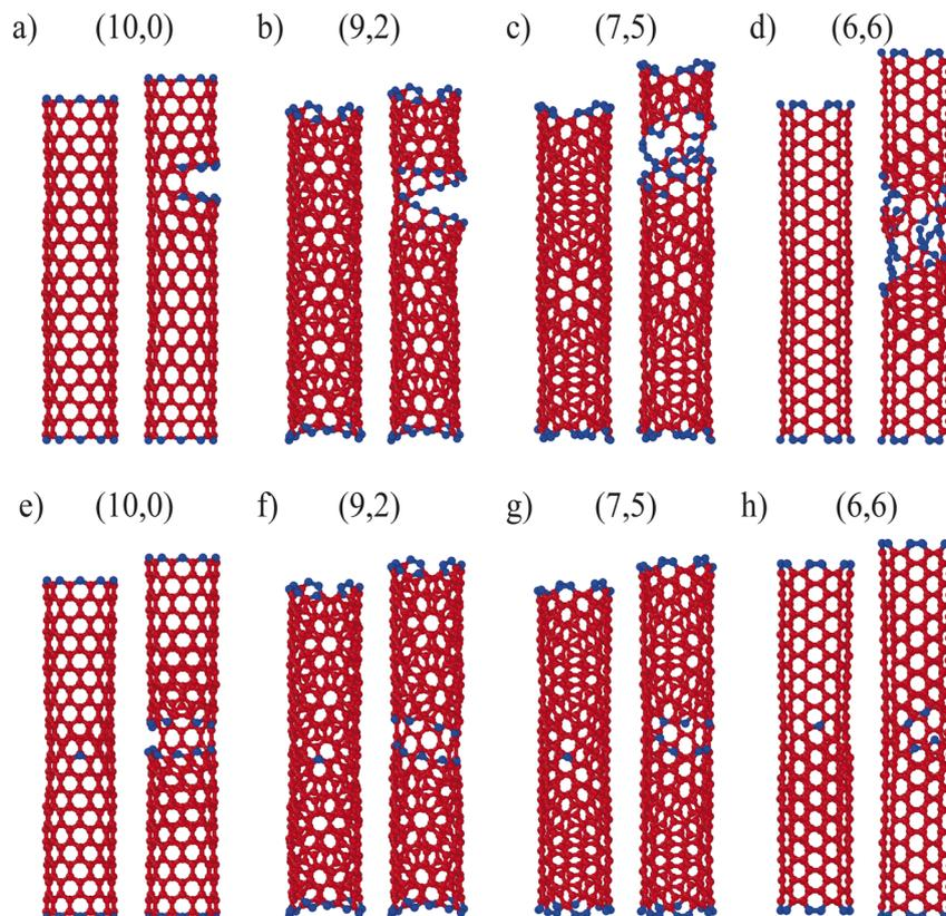
Fig. 2 Illustration of (a–d) pristine and (e–h) defective carbon nanotubes (CNTs) with varying chiral angles and similar diameters. The figure on the left of each pair shows the structure before applying any strain, and the right figure shows the structure after the fracture occurs. The chiral indices of each CNT are mentioned above each pair. The blue and red spheres represent carbon atoms with coordination numbers of 2 and 3, respectively.
