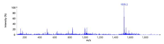
Fig. 2 High-resolution mass spectrometry (HRMS) ESI of (A) surfactin ( $C_{53}H_{93}N_7O_{13}$ ) showing the main m/z (M + H) at 994.6, 1008.5, 1022 and 1036.7 (B) OleSurf ( $C_{89}H_{163}N_9O_{11}$ ) calc. 1535 found 1535.2.
