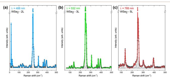
Fig. 4 Lorentzian deconvolution of the Raman spectra for (a) 2L WSe<sub>2</sub> measured at 488 nm, (b) 3L WSe<sub>2</sub> measured at 532 nm and (c) 5L WSe<sub>2</sub> measured at 785 nm excitation wavelengths.
