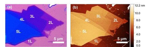
Fig. 1 Morphological characterization of a  $WSe_2$  flake on a  $SiO_2/Si$  substrate. (a) Optical microscopy image showing different contrasts within the  $WSe_2$  flake attributed to different numbers of layers: monolayer (1L), bilayer (2L), three-layer (3L), four-layer (4L) and five-layer (5L). (b) AFM image of the  $WSe_2$  flake measured in tapping-mode showing the height profile and confirming the assignment of the different numbers of layers.
