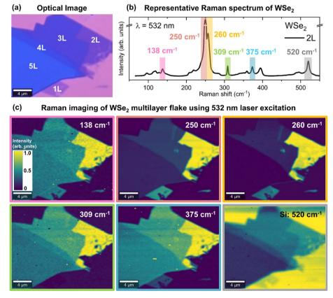
Fig. 2 Raman imaging of the multilayer  $WSe_2$  flake. (a) Optical image of the flake using a Raman microscope. (b) Representative spectrum of the  $WSe_2$  flake recorded on the bilayer area using an excitation wavelength of 532 nm. The main peaks are highlighted on the spectrum and their respective intensities over the flake are shown in the Raman images in (c).
