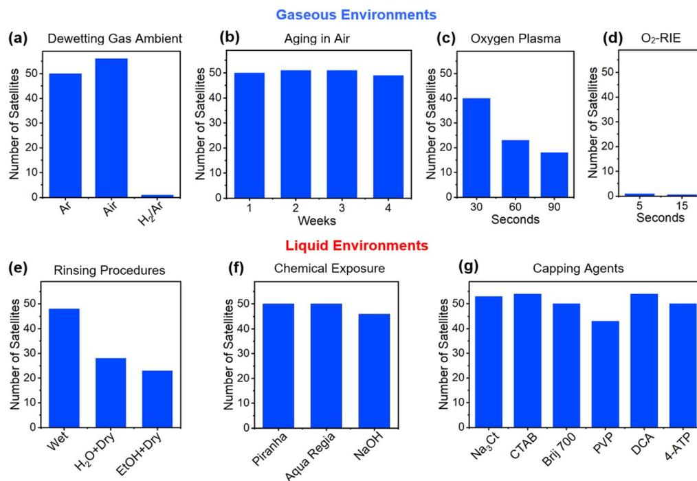
Fig. 3 Histograms showing satellite attachment to cores that were (a) assembled in various gas ambients, (b) aged in air, (c) cleaned in an O<sub>2</sub> plasma, (d) exposed to an O<sub>2</sub>-RIE treatment, (e) rinsed in different manners after dithiol attachment, (f) exposed to cleaning solutions, and (g) functionalized with various capping agents.
