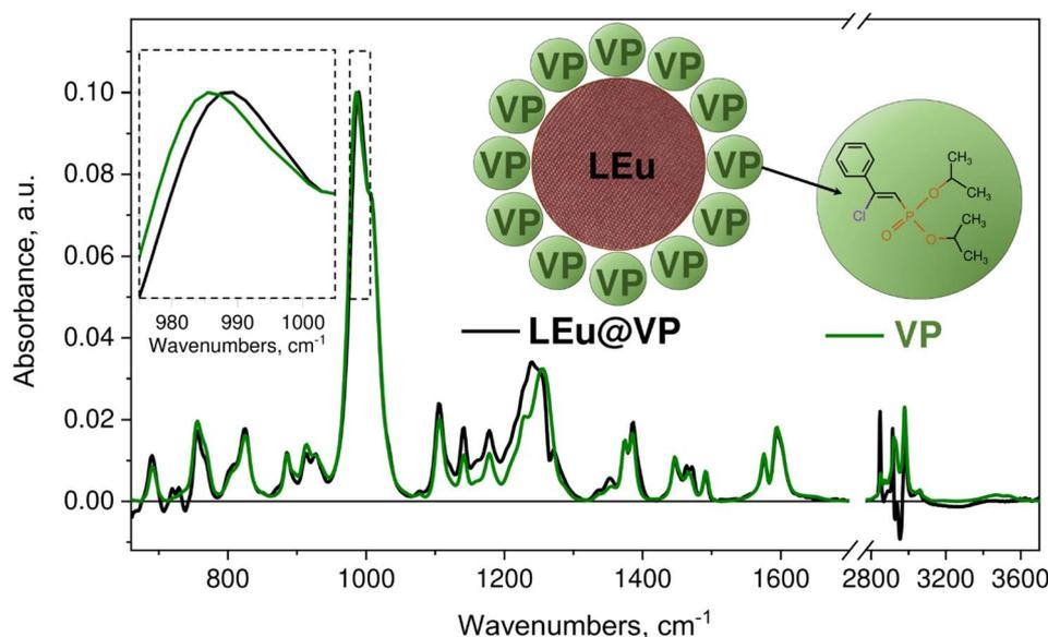
Fig. 1 Schematic representation of hybrids  $\text{LEu@VP}$  and absorbance spectrum of VP solution in dichloromethane with subtraction of solvent contribution (green) and absorbance spectrum of hybrids  $\text{LEu@VP}$  solution in dichloromethane with subtraction of solvent and LEu contributions (black).
