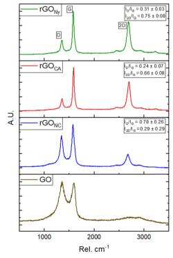
Fig. 3 Raman spectra of rGO film in each membrane used as substrate compared to the GO Raman spectra.
