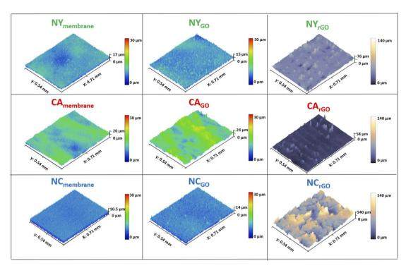
Fig. 2 3D models of surface characterization of each sample by confocal laser scanning microscopy. Surface images of pure membrane (1st column), GO surface (2nd column), and rGO surface (3rd column) obtained with photoreduction process using OS1. Membranes: Nylon (Ny) in green, Cellulose Acetate (CA) in red, and Nitrocellulose (NC) in blue.
