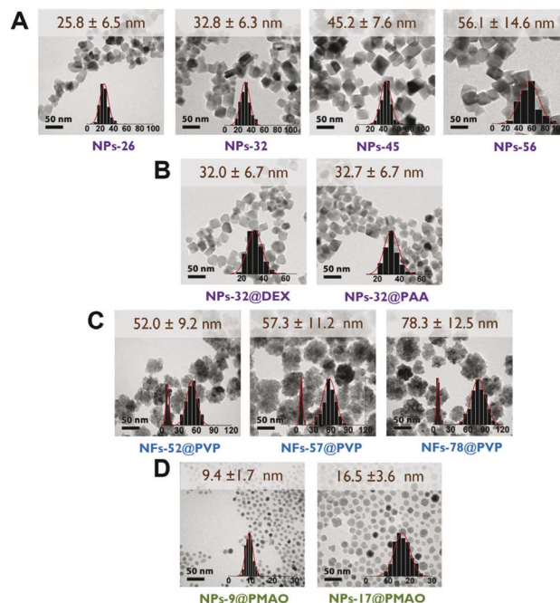
Fig. 1 TEM images and particle size distribution: (group A) uncoated octahedral nanoparticles with sizes between 26 and 56 nm, (group B) 32 nm octahedral nanoparticles with different coatings, (group C) nanoflowers with the same core size (8–10 nm) and coating (polyvinylpyrrolidone) and different particle sizes (52–78 nm), and (group D) spherical nanoparticles with sizes of about 9 and 17 nm coated with PMAO.
