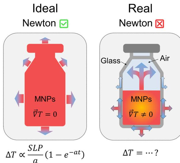
Fig. 2 Schematic illustration of the differences between the ideal scenario under which Newton's law of cooling would be applicable (*i.e.* homogeneous temperature, and one heat-exchange mechanism; left panel); and the real situation in which the sample temperature is not homogeneous, and heat can be exchanged through different channels (right panel).
