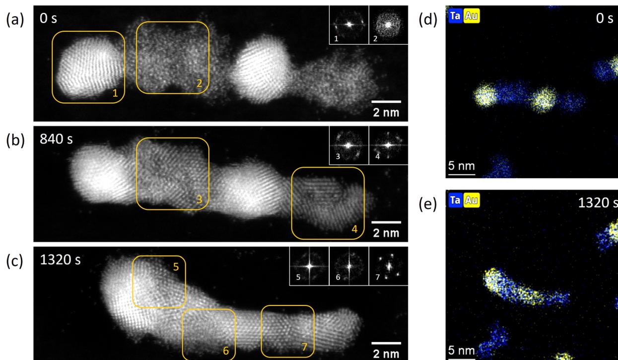
Fig. 5 (a–c) Electron beam welding of Au<sub>923</sub>–Ta<sub>923</sub>–Ta<sub>923</sub>–Au<sub>923</sub>–Ta<sub>923</sub> chain of clusters. The corresponding EDS elemental mappings are shown in (d) and (e) respectively.
