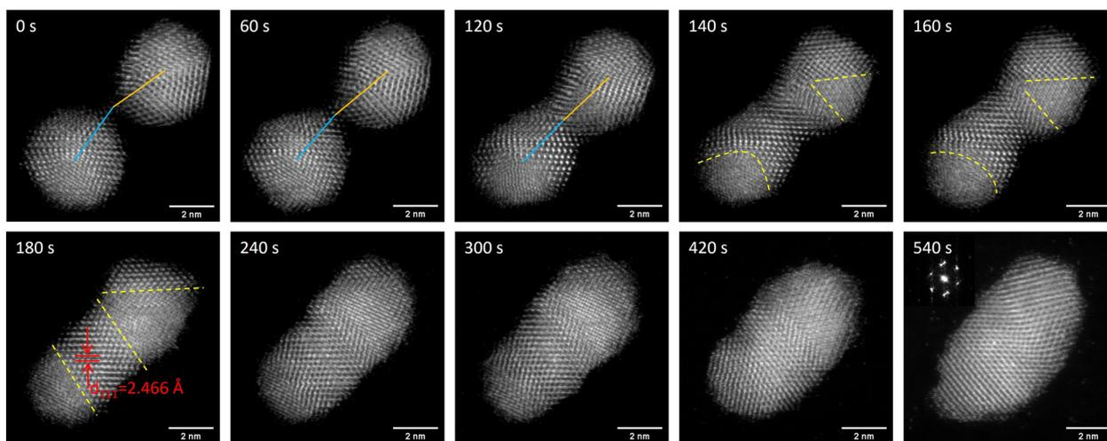
Fig. 1 Real-time sequential HAADF-STEM images of the coalescence process of Au<sub>2057</sub> clusters under electron beam irradiation. The blue and orange lines connect the center of Au<sub>2057</sub> clusters to the center of the neck, while the yellow dashed lines represent grain boundaries. The inset at 540 s shows the corresponding FFT power spectrum.
