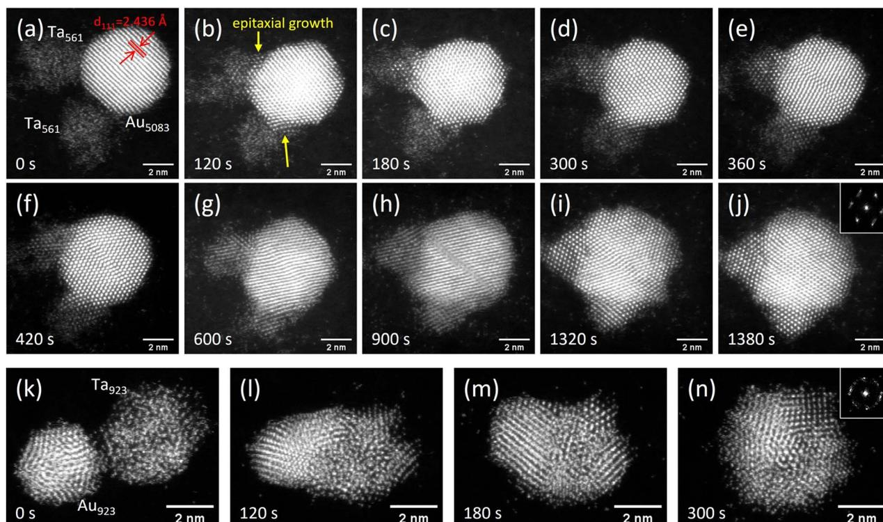
Fig. 4 (a–j) The EBW between two amorphous Ta<sub>561</sub> clusters and one FCC-structured Au<sub>5083</sub> cluster. (k–n) The EBW between distorted decahedral Au<sub>923</sub> cluster and amorphous Ta<sub>923</sub> cluster. The insets in (j) and (n) show the corresponding FFT power spectrum.
