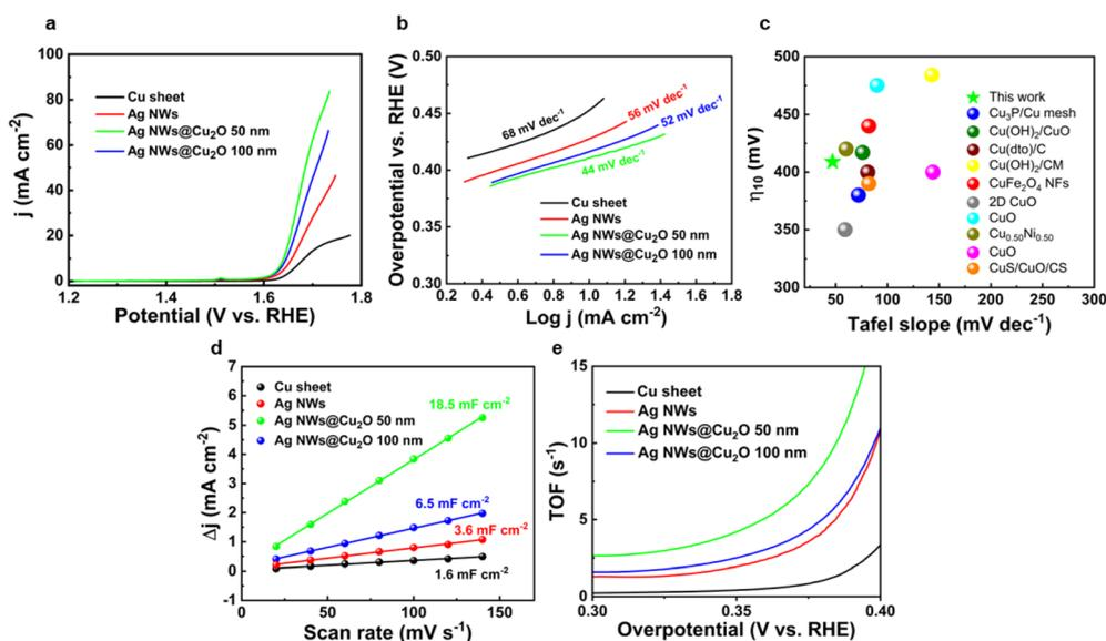
Fig. 5 OER performance of various coatings grown on Cu sheet in 1 M KOH. (a) Polarization curves, (b) corresponding Tafel plots, (c) comparison of  $\eta_{10}$  and Tafel slopes of some recent representative reports of copper-based OER catalysts, (d) current density plots, and (e) TOF plots.
