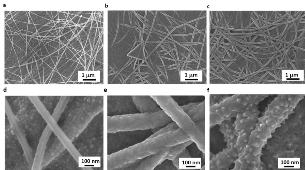
Fig. 3 Morphological analysis of various coatings deposited on Cu sheet. Low and high magnification SEM images of (a and d) bare AgNWs, (b and e) AgNWs@50 nm-thick  $\text{Cu}_2\text{O}$ , and (c and f) AgNWs@100 nm-thick  $\text{Cu}_2\text{O}$ .
