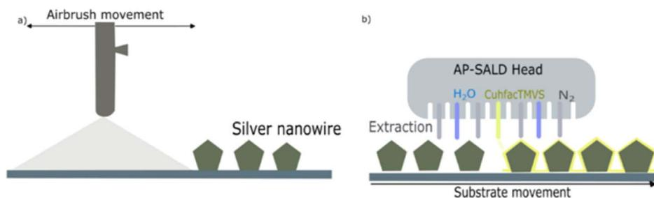
Fig. 1 Schematic illustration of the deposition process for (a) AgNW networks, and (b)  $\text{Cu}_2\text{O}$  thin films to fabricate AgNW@ $\text{Cu}_2\text{O}$  nanocomposite networks (note that this drawing is not to scale).
