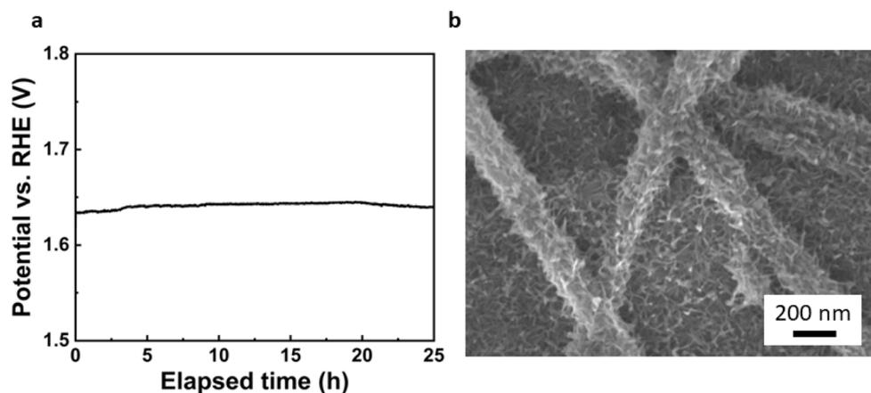
Fig. 6 (a) Chronopotentiometric curve and (b) SEM after OER of AgNWs@ 50 nm-thick Cu<sub>2</sub>O.
