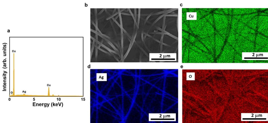
Fig. 4 (a) EDX spectrum of AgNWs/50 nm-thick  $\text{Cu}_2\text{O}$ . (b–e) SEM image and the corresponding elemental maps of AgNWs@50 nm-thick  $\text{Cu}_2\text{O}$ .
