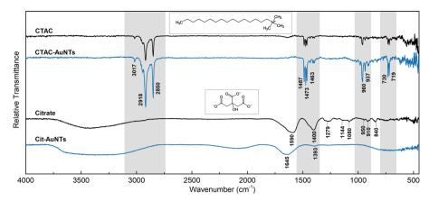
Fig. 6 Relative vacuum transmittance FTIR spectra of CTAC- and citrate-capped nanotriangles (blue lines), and the reference spectra of the pure ligands (black lines). The characteristic modes in the CTAC molecule are highlighted in grey.
