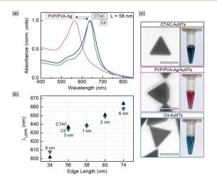
Fig. 4 UV–VIS spectra (a) for 58 nm AuNTs during the indirect ligand exchange process. The LSPR peak positions (b) show the shift after the ligand exchange for the samples with various edge lengths (34, 56, 58, 65, and 74 nm as indicated by the *X*-axis). STEM micrographs of 58 nm AuNTs (c) reveal the morphology change at the intermediate step; scale bars are 50 nm.
