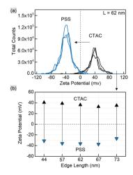
Fig. 2 Zeta-potential measurements for CTAC- and PSS-capped AuNTs. The representative curves (a) are given for the 62 nm nanotriangles. The graph (b) shows the respective peak positions for AuNTs with various edge lengths (44, 57, 62, 67, and 73 nm as indicated by the *X*-axis).
