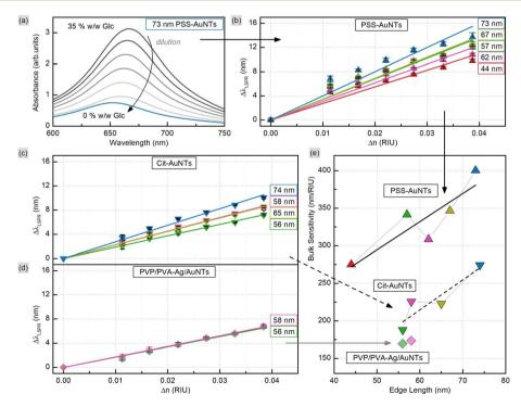
Fig. 7 Determination of bulk sensitivity (e) based on the plasmonic shift  $(\Delta \lambda_{LSPR})$  as a response to the change in the refractive index of the medium  $(\Delta n)$  upon glucose addition (a) to AuNTs with various dimensions and surface ligands (b-d).
