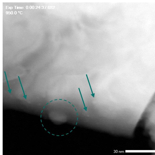
Fig. 5 *In situ* STEM-ADF image of the L1.85NTR sample measured at 950 °C in high vacuum. The green arrows highlight the exsolved nanoparticles/nuclei with smaller size.
