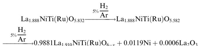
However, precisely determining the oxygen stoichiometry of the resulting  $\text{La}_{1.910}\text{NiTi}_{0.9}\text{Ru}_{0.1}\text{O}_{6-y}$  double perovskite remains challenging due to the uncertainty surrounding the exsolution behaviour of Ni cations or Ni–O species.
