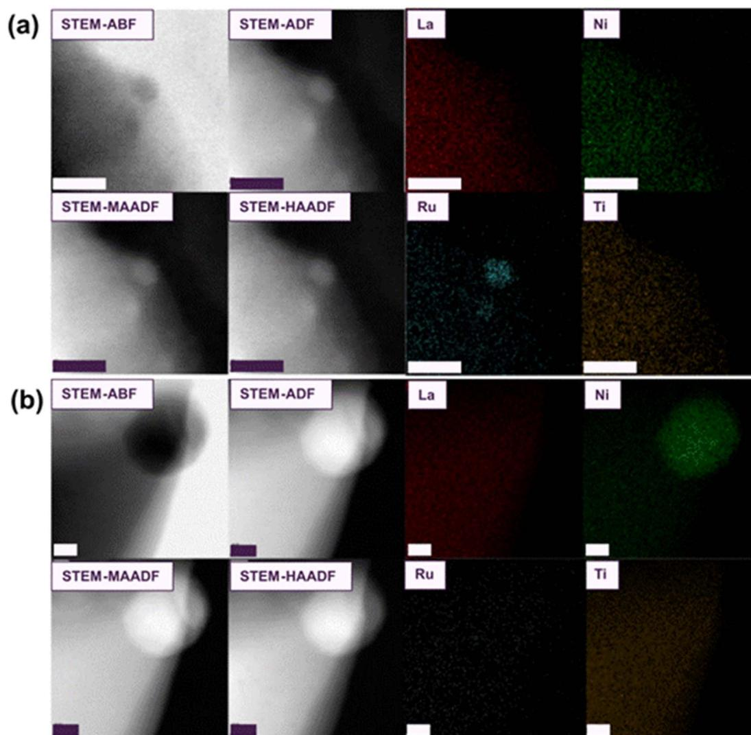
Fig. 3 STEM images and EDX maps of two distinct regions (a) and (b) of the L1.85NTR sample reduced at 1000 °C in a wet 5% H<sub>2</sub>/Ar for 3 hours. Scale bar: (a) 5 nm; (b) 10 nm.
