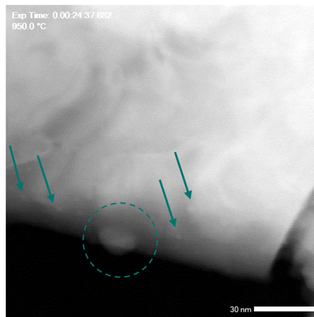
Fig. 5 In situ STEM-ADF image of the L1.85NTR sample measured at 950^\circ\text{C} in high vacuum. The green arrows highlight the exsolved nanoparticles/nuclei with smaller size.
