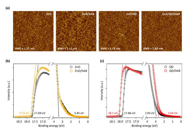
Fig. 2 (a) Atomic force microscopy (AFM) images of ZnO film, ZnO film with DAB treatment, QD film and QD film with DAB treatment (5  $\mu$ m  $\times$  5 μm). Ultraviolet photoelectron spectroscopy (UPS) spectra of (b) ZnO and (c) QD films with and without DAB treatment.
