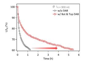
Fig. 5 Lifetime measurement of the QD-LEDs with and without DAB ligands at an initial luminance of 900 nit. The measurement was performed in ambient air without any type of passivation or encapsulation.
