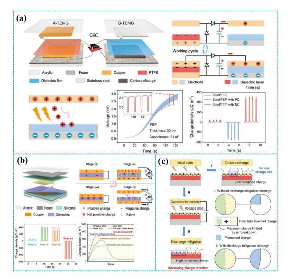
Fig. 9 (a) Structure and principle of charge injection enabled by air breakdown achieved by a half-wave charge excitation circuit. Reprinted with permission from ref. 50. Copyright 2022, Wiley. (b) Theory analysis for the charge reversion process. Reprinted with permission from ref. 37. Copyright 2023, Royal Society of Chemistry. (c) Discharge mitigation strategy to decrease the dissipation of the injected surface charge. Reprinted with permission from ref. 141. Copyright 2023, Wiley.
