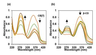
Fig. 4 UV-Vis titration spectra of (a) AVO (0.04 mM) in the presence of CB[7] (0–2 mM) in 10% ethanol and (b) AVO (0.04 mM) in the presence of  $\beta$ -CD (0–4 mM) in 10% ethanol.
