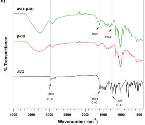
Fig. 5 FTIR spectra of (a) (top to bottom) the AVO–CB[7] complex (1: 1) prepared by the kneading method, CB[7], and AVO; (b) (top to bottom) the AVO– $\beta$ -CD complex (1:1) prepared by the solvent evaporation method,  $\beta$ -CD, and AVO.
