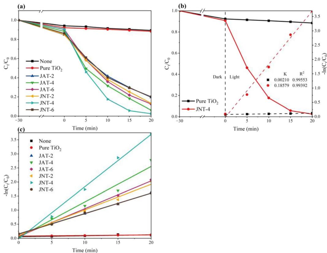
Fig. 11 Photocatalytic degradation (a) and the corresponding  $-\ln(C_t/C_0)$  variations (b and c) of RhB with JAT, JNT nanocrystals, pure  $\text{TiO}_2$  and without photocatalysts under a mercury lamp ( $\lambda \geq 400$  nm).
