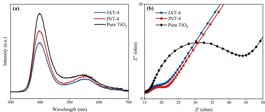
Fig. 10 PL spectrum (a) and Nyquist plot (b) of JAT-4, JNT-4 nanocrystals and pure TiO<sub>2</sub>.
