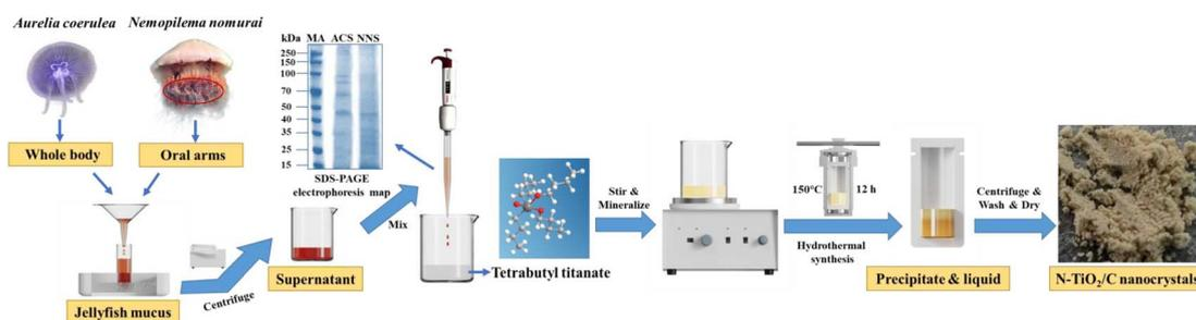
Fig. 1 Schematic of the synthetic process of nitrogen-doped TiO<sub>2</sub> nanocrystals modified with carbon (N-TiO<sub>2</sub>/C) by using proteins of the large harmful jellyfish *Aurelia coerulea* and *Nemopilema nomurai* mucus as dopants (MA: marker, ACS: *A. coerulea* mucus, NNS: *N. nomurai* mucus).
