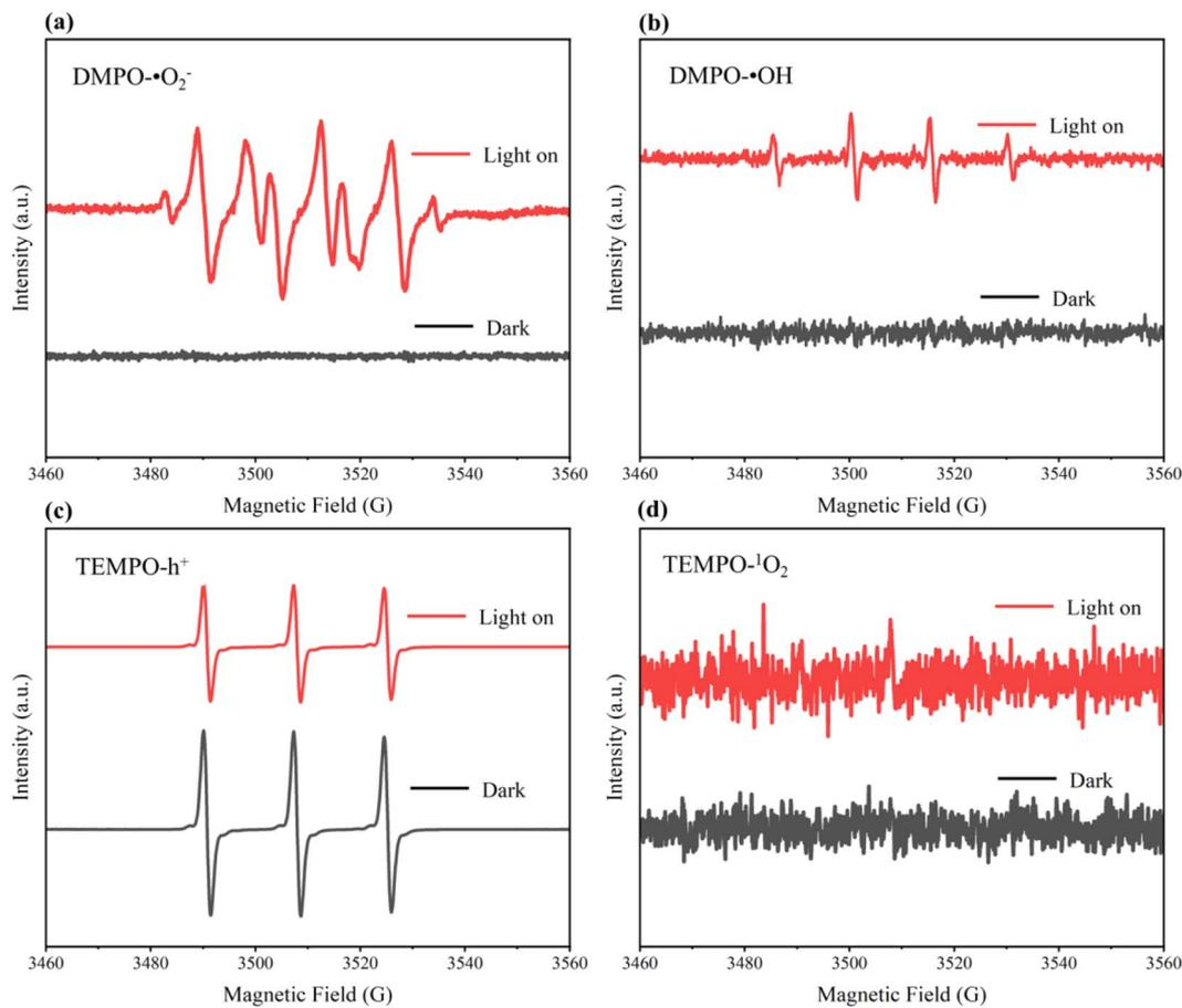
Fig. 13 ESR spectra of DMPO- $\cdot\text{O}_2^-$  (a), DMPO- $\cdot\text{OH}$  (b), TEMPO- $\text{h}^+$  (c) and TEMPO- $^1\text{O}_2$  (d) of JNT-4 nanocrystals in the dark and under mercury lamp ( $\lambda \geq 400$  nm) irradiation.
