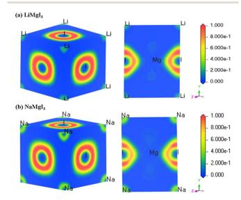
Fig. 3 DFT-computed electron localization function (ELF) in the 3D and 110 crystal direction of (a) LiMgl<sub>3</sub> and (b) NaMgl<sub>3</sub> single perovskite compounds, respectively.
