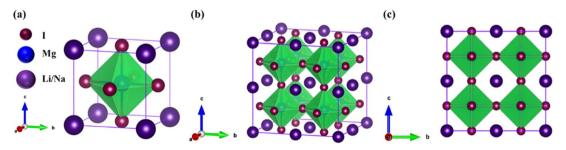
Fig. 1 Optimized crystal structure of  $XMgI_3$  (X = Li/Mg) halide-based single perovskite compounds: (a) 3D unit cell, (b) 3D, and (c) 2D supercell (2  $\times$  2  $\times$  2). The purple-color ball represents a Li or Na atom, the blue-color ball represents an Mg atom, and the dark-purple color represents an I atom.
