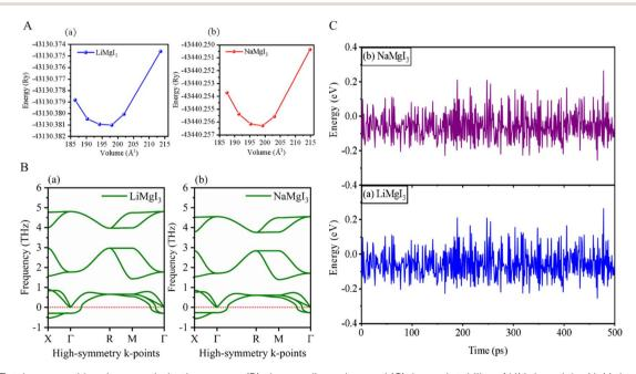
Fig. 2 (A) Total energy with volume optimization curves, (B) phonon dispersion, and (C) thermal stability of  $LiMgl_3$  and the  $NaMgl_3$ , respectively.
