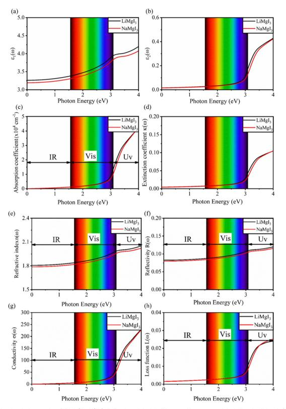
Fig. 7 Calculated optical properties of XMgI<sub>3</sub> (X = Li/Na) alkaline-based single halide perovskite compounds including the dielectric functions for (a) real part  $(\epsilon_1(\omega))$ , (b) imaginary part  $(\epsilon_2(\omega))$ , (c) absorption coefficient  $(\alpha(\omega))$ , (d) extinction coefficient  $(k(\omega))$ , (e) index of refraction  $(n(\omega))$ , (f) reflectivity  $(R(\omega))$ , (g) conductivity  $(\sigma(\omega))$ , and (h) loss function  $(L(\omega))$ .
