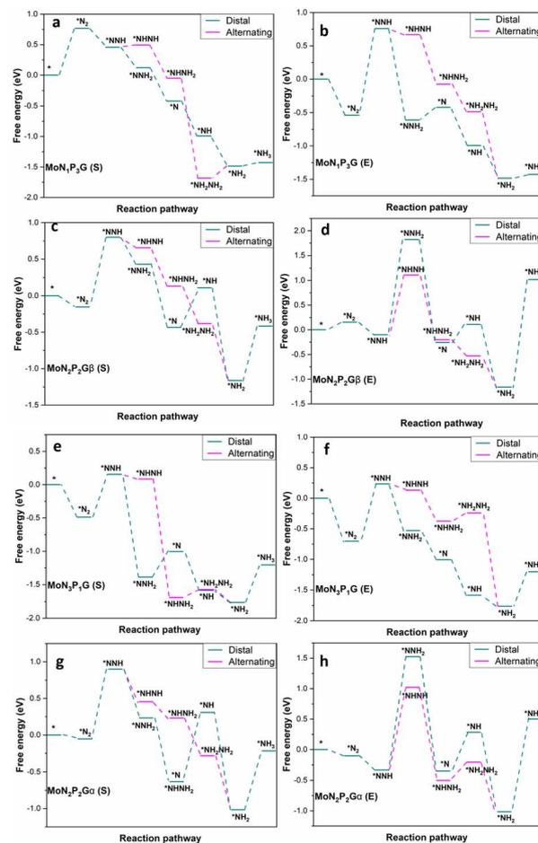
Fig. 2 Distal and alternating routes for the NRR on  $\text{MoN}_3\text{P}_1\text{G}$ ,  $\text{MoN}_2\text{P}_2\text{G}\beta$ ,  $\text{MoN}_3\text{P}_1\text{G}$  and  $\text{MoN}_2\text{P}_2\text{G}\alpha$  catalysts with  $\text{N}_2$  end-on (E) and side-on (S) adsorption.
