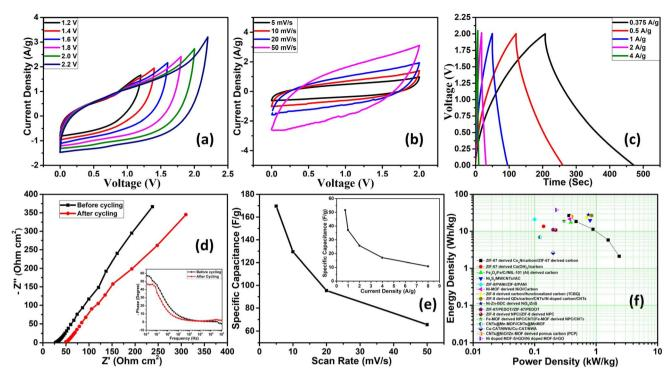
Fig. 6 Electrochemical characterization of the asymmetrical device (Co<sub>4</sub>N/carbon//Z-800): (a) voltage window test, (b) CV at different scan rates, (c) GCD at different current densities, (d) Nyquist plot (inset: phase vs. frequency), (e) capacitance vs. scan rate (inset: capacitance vs. current density), and (f) Ragone plot
