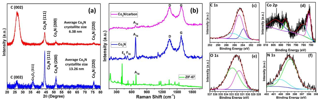
Fig. 2 (a) XRD pattern of  $\text{Co}_4\text{N}$  bulk (blue line) and  $\text{Co}_4\text{N}/\text{carbon}$  (red line) and (b) Raman spectra of ZIF-67, bulk  $\text{Co}_4\text{N}$ , and  $\text{Co}_4\text{N}/\text{carbon}$ ; high resolution XPS spectra of (a) C 1s, (b) Co 2p, (c) O 1s, and (d) N 1s.
