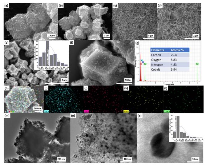
(a and b) Z-800 FESEM, (c and d) bulk Co<sub>4</sub>N FESEM, (e) FESEM of Co<sub>4</sub>N/carbon (inset: carbon structure size distribution), (f) single Co<sub>4</sub>N/ carbon structure FESEM, (g) EDS of  $Co_4N$ /carbon (inset: elemental composition), (h-l) elemental mapping of  $Co_4N$ /carbon single particle, (m and n) TEM image of  $Co_4N$ /carbon, (o) high resolution TEM of the  $Co_4N$  nanoparticle in the carbon structure (inset:  $Co_4N$  particle size distribution).
