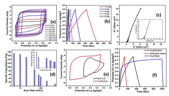
Fig. 4 (a) CV analysis of  $Co_4N$ /carbon at different scan rates, (b) GCD of  $Co_4N$ /carbon at different current densities, (c) Nyquist plot (inset: enlarged view of the Nyquist plot), (d) capacitance vs. scan rate (inset: capacitance vs. current density), (e) CV comparison of bulk  $Co_4N$  and  $Co_4N$ /carbon, and (f) GCD comparison of  $Co_4N$ /carbon, bulk  $Co_4N$ , and activated carbon.
