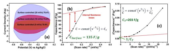
Fig. 5 (a) Surface controlled contribution CV curve of  $Co_4N$ /carbon at 5 mV s<sup>-1</sup>, 10 mV s<sup>-1</sup>, and 20 mV s<sup>-1</sup>. (b) Variation of specific capacitance with inverse of square root of scan rate to evaluate maximum surface controlled contribution and (c) variation of inverse of specific capacitance with square root of scan rate to evaluate total possible capacitance including surface controlled and diffusion controlled current.
