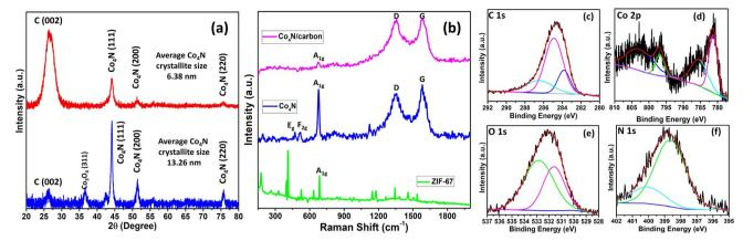
Fig. 2 (a) XRD pattern of  $Co_4N$  bulk (blue line) and  $Co_4N$ /carbon (red line) and (b) Raman spectra of ZIF-67, bulk  $Co_4N$ , and  $Co_4N$ /carbon; high resolution XPS spectra of (a) C 1s, (b) Co 2p, (c) O 1s, and (d) N 1s.
