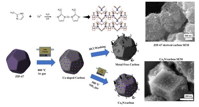
Fig. 1 Synthesis scheme of the Co<sub>4</sub>N/carbon and Z8-800 (metal free carbon).
