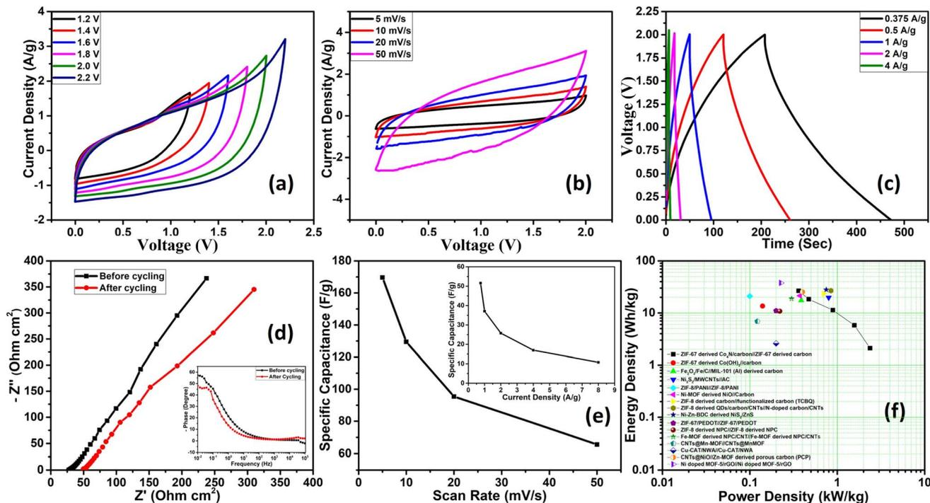
Fig. 6 Electrochemical characterization of the asymmetrical device ( $\text{Co}_4\text{N}/\text{carbon}/\text{Z}-800$ ): (a) voltage window test, (b) CV at different scan rates, (c) GCD at different current densities, (d) Nyquist plot (inset: phase vs. frequency), (e) capacitance vs. scan rate (inset: capacitance vs. current density), and (f) Ragone plot.
