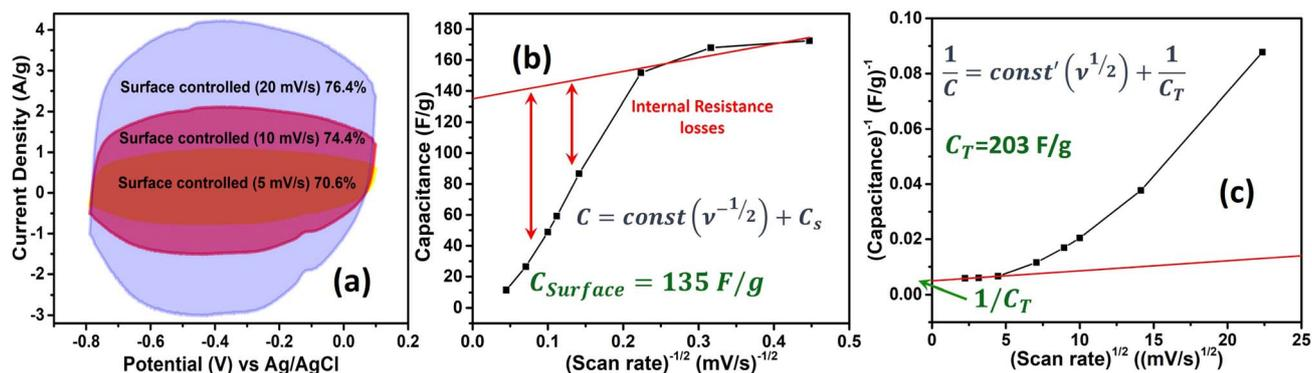
Fig. 5 (a) Surface controlled contribution CV curve of  $\text{Co}_4\text{N}/\text{carbon}$  at  $5 \text{ mV s}^{-1}$ ,  $10 \text{ mV s}^{-1}$ , and  $20 \text{ mV s}^{-1}$ . (b) Variation of specific capacitance with inverse of square root of scan rate to evaluate maximum surface controlled contribution and (c) variation of inverse of specific capacitance with square root of scan rate to evaluate total possible capacitance including surface controlled and diffusion controlled current.
