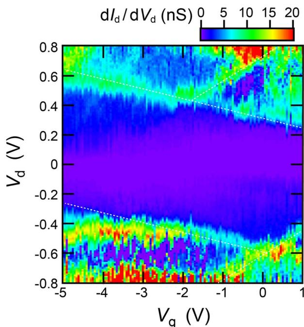
Fig. 4 Experimental  $V_d$ - $V_g$  2D  $dI_d/dV_d$  plot. The Coulomb diamond is outlined with white dotted lines.
