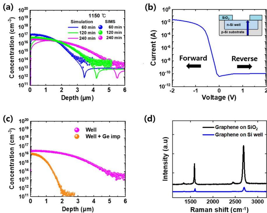
Fig. 2 (a) Dopant profiles of phosphorus in the p-Si substrate (solid line: simulated data, scattered dot: real SIMS measurement data). Each dopant profile had different annealing time for activation. (b) PN junction leakage current measurement (p-Si substrate/n-Si well junction). (c) SIMS profiles after Ge ion implantation (d) Raman spectrum of transferred monolayer graphene on SiO<sub>2</sub>, Si well.
