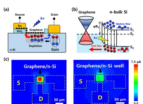
Fig. 4 (a) Cross-sectional schematic of the graphene/n-type bulk Si photodetector. (b) The energy band diagram of a graphene/n-type bulk Si photodetector under illumination conditions. (c) Scanning photocurrent microscopy image of the graphene/n-type bulk Si photodetector (left) and graphene/n-Si well-tub/p-Si photodetector (right), both presented on the same scale. The black dashed areas indicate the junction of graphene and Si ( $V_d = -0.5 \text{ V}$ ,  $\lambda = 850 \text{ nm}$ ).
