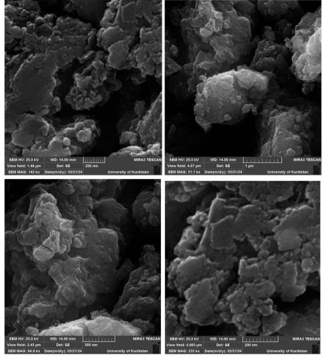
Fig. 9 SEM images of recycled Cu-P.bis(OA)@FeB-MNPs catalyst.
