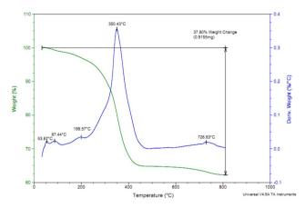
Fig. 4 TGA/DTG diagrams for Cu-P.bis(OA)@FeB-MNPs.
