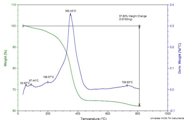
Fig. 4 TGA/DTG diagrams for Cu-P.bis(OA)@FeB-MNPs.
