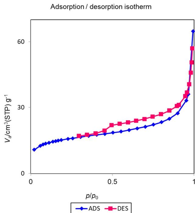
Fig. 5 N<sub>2</sub> adsorption–desorption isotherms of Cu-P.bis(OA)@FeB-MNPs.
