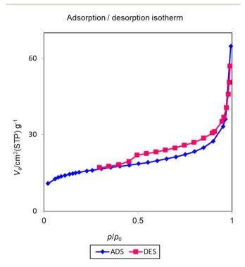
Fig. 5  $N_2$  adsorption–desorption isotherms of Cu-P.bis(OA)@FeB-MNPs.
