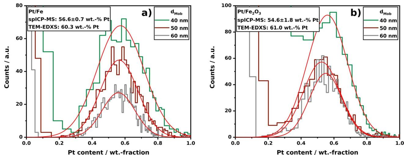
Fig. 5 Composition distributions of Pt/Fe (a) and Pt/Fe<sub>2</sub>O<sub>3</sub> (b) aerosol NPs sintered at 1000 °C obtained by spICP-MS. For each indicated size fraction,  $n = 1000 \pm 50$  single-particles were analyzed. The red Gaussian fits act as a guide to the eye. spICP-MS raw data are depicted in Fig. S4 and S5.†
