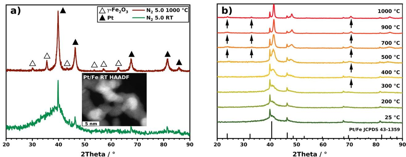
Fig. 6 X-ray diffractograms of (a) Pt/Fe at room temperature (RT) and sintered under N<sub>2</sub> at 1000 °C. The inset shows the HAADF image of Pt/Fe NPs at room temperature indicating the crystalline structure of Pt in primary particles. (b) Pt/Fe sintered under H<sub>2</sub> at different temperatures. Reference reflexes are given for Pt/Fe in L1<sub>0</sub> configuration and additionally indicated by arrows.
