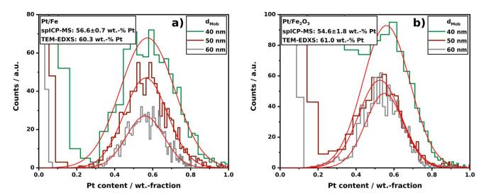
Fig. 5 Composition distributions of Pt/Fe (a) and Pt/Fe<sub>2</sub>O<sub>3</sub> (b) aerosol NPs sintered at 1000 °C obtained by spICP-MS. For each indicated size fraction,  $n = 1000 \pm 50$  single-particles were analyzed. The red Gaussian fits act as a guide to the eye. spICP-MS raw data are depicted in Fig. S4 and S5  $\dot{\tau}$
