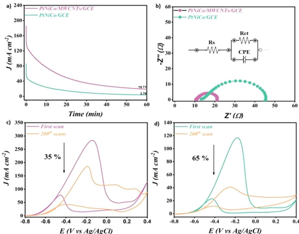
Fig. 6 (a) Chronoamperometric curves for PtNiCo and PtNiCo/MWCNTs in  $1$  M KOH solution containing  $1$  M CH $_3$ OH. (b) Nyquist plots for PtNiCo and PtNiCo/MWCNTs in  $1$  M KOH solution containing  $1$  M CH $_3$ OH at  $-0.3$  V. (c and d) Long term durability test for PtNiCo/MWCNTs, and PtNiCo.
