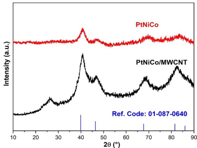
Fig. 1 XRD patterns of the PtNiCo and PtNiCo/MWCNT electrocatalysts.
