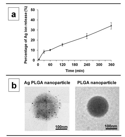
Fig. 1 (a) Percentage of silver ions released from Ag PLGA nanoparticles at 5, 30, 60, 120, 240, and 360 min. (b) TEM images of an Ag PLGA nanoparticle and PLGA nanoparticle.
