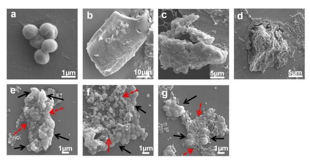
Fig. 2 SEM images of (a) the *S. epidermidis* bacterial cells, (b) biofilms without any treatment, and the biofilms treated with Ag PLGA nanoparticles immediately (c), and after (d) 30 min, (e) 2 h, (f) 4 h, and (g) 6 h. The black and dashed red arrows indicate bacterial cells and Ag PLGA nanoparticles.
