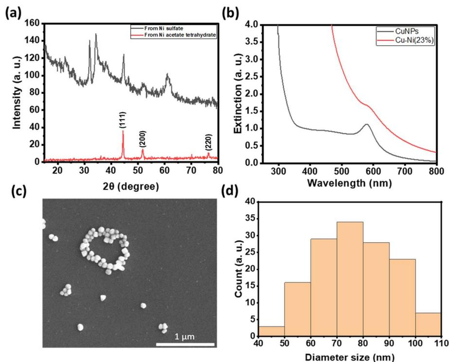
**Fig. 3** (a) X-ray diffraction patterns of metallic nickel synthesized from nickel acetate tetrahydrate (top red) and mixed nickel hydroxide and oxide from nickel sulfate (bottom black). (b) UV-vis extinction spectrum of as-synthesized CuNPs and Cu-Ni NPs. (c) SEM image of Cu-Ni NPs and (d) their size distribution ( $N = 126$ ).
