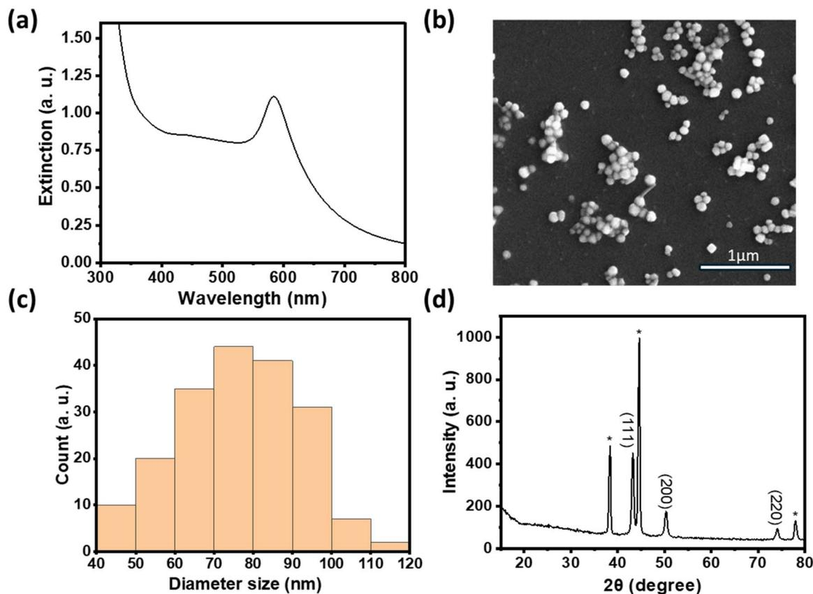
Fig. 1 (a) UV-vis extinction spectrum of as-synthesized CuNPs. (b) SEM image of CuNPs and (c) their size distribution ( $N = 175$ ). (d) XRD pattern of purified CuNPs (peaks labeled with \* came from the sample holder).
