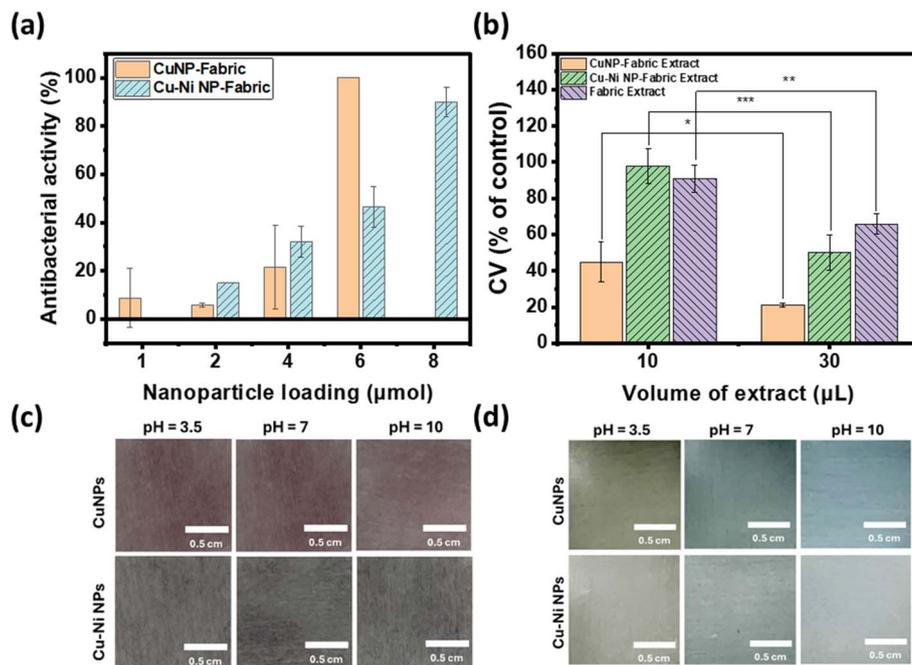
Fig. 5 (a) Antibacterial activity of different amounts of CuNP- or Cu-Ni NP-coated fabrics. (b) Cell viability after incubation with extracts of CuNP- and Cu-Ni NP-coated fabrics. \*:  $p < 0.05$ . \*\*:  $p < 0.01$ . \*\*\*:  $p < 0.001$ . Photographs of CuNP- and Cu-Ni NP-coated fabrics in SWE with different pHs (c) at the beginning and (d) after 105 min of incubation.
