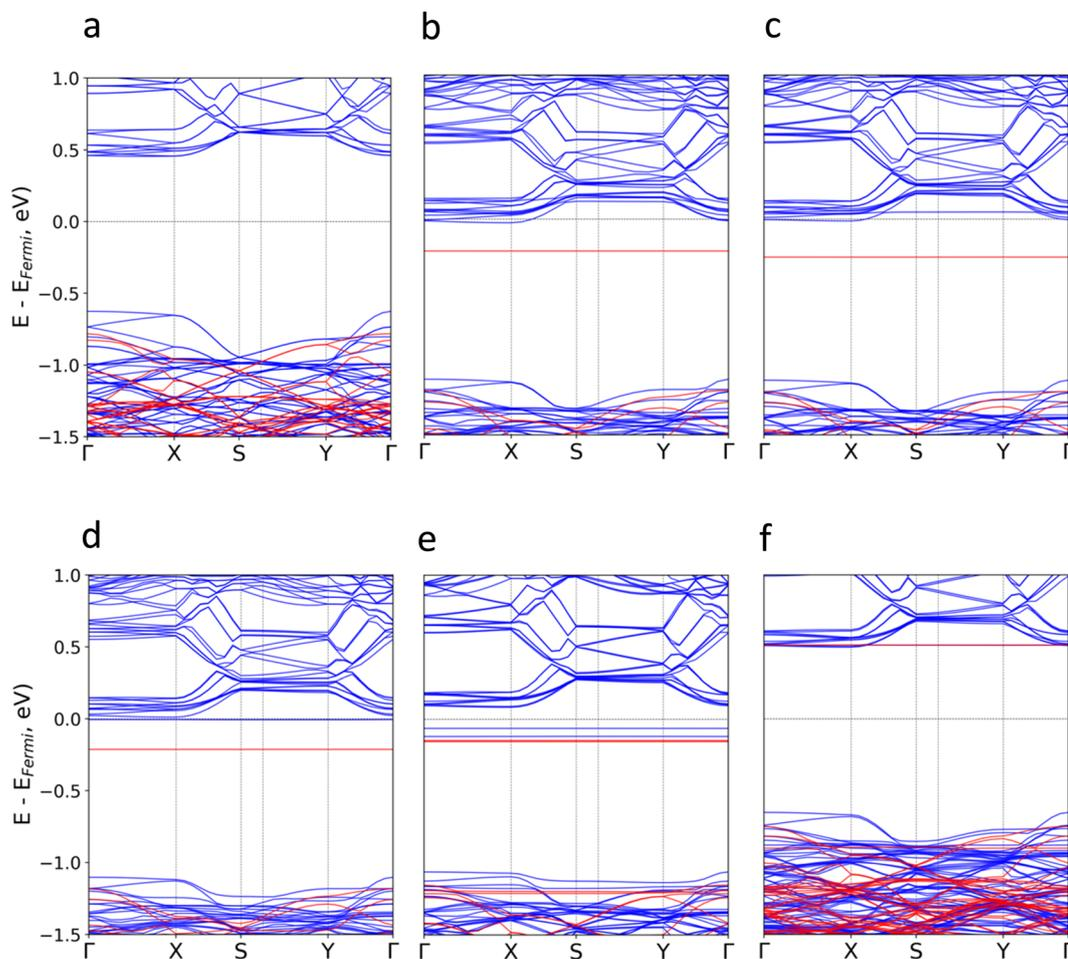
Fig. 3 Calculated electronic band structure for (a) pristine CrSBr and the hybrid molecular/2D heterostructures based on (b) TTF-CH<sub>3</sub>, (c) TTF, (d) perylene, (e) coronene, (f) TCNQ. Blue (red) colour represents spin up (down) energy bands.
