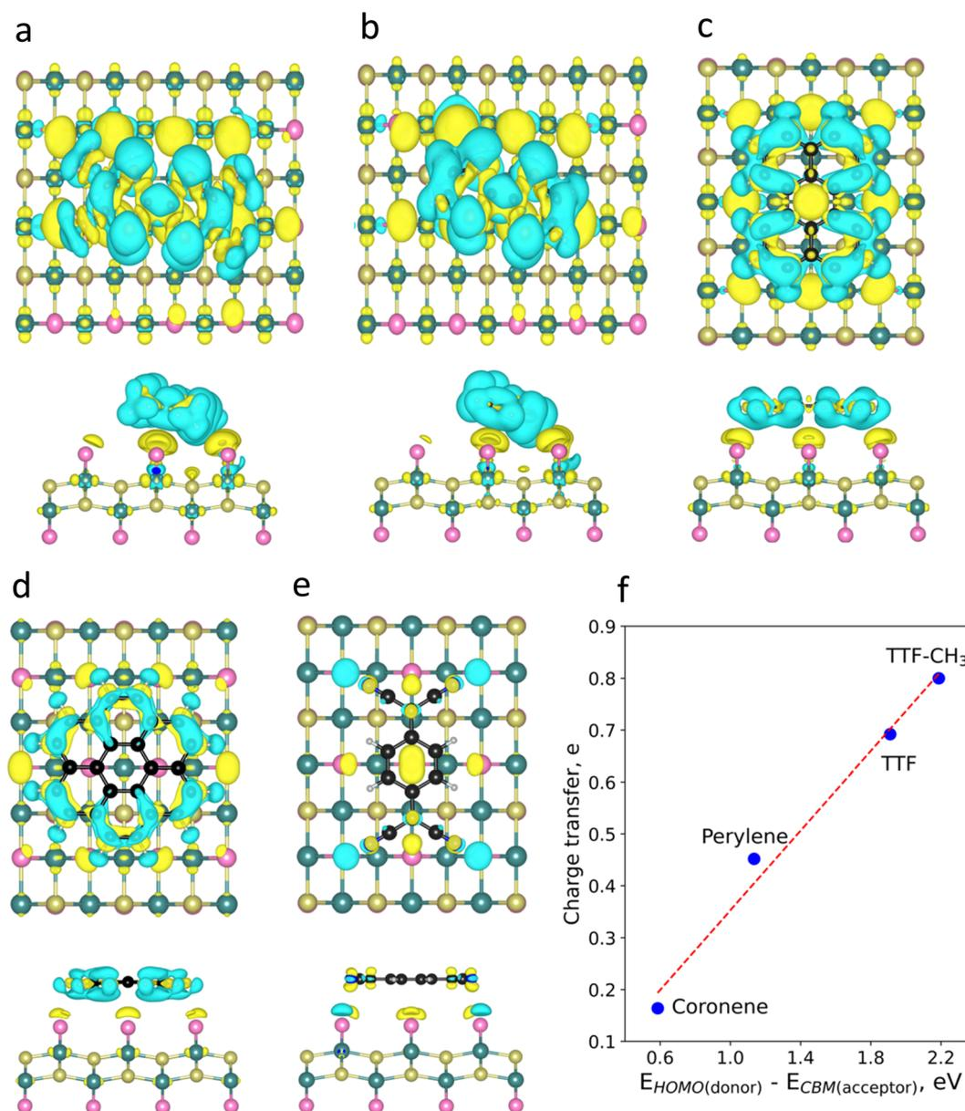
Fig. 2 Charge density difference (CDD) plots of (a) TTF-CH<sub>3</sub>, (b) TTF, (c) perylene, (d) coronene, and (e) TCNQ. Blue and yellow colours represent regions with charge depletion and accumulation, respectively. (f) Evolution of charge transfer with the energy difference between the HOMO of the donor molecules and CBM of CrSBr.
