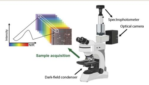
Fig. 1 The components of an HSI system (right) and HSI data cube (left).
