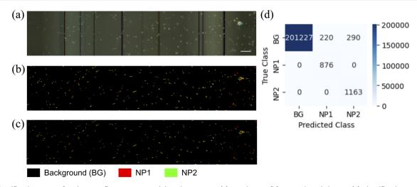
Fig. 6 Classification maps for the two fluorescent particle mixture case (a) raw image (b) ground truth image (c) classification result (d) the confusion matrix for our result.
