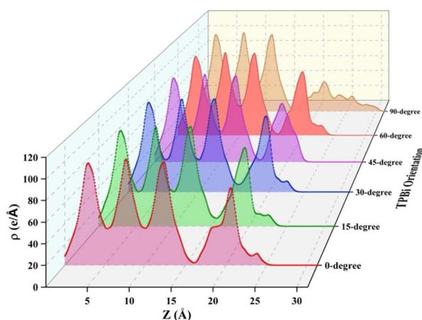
Fig. 6 Charge density of TPBi-(PEA)<sub>2</sub>PbI<sub>4</sub> interfaces.
